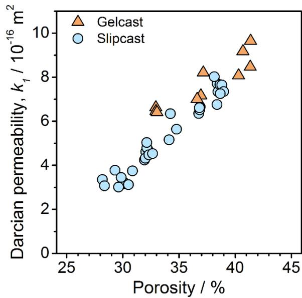
Fig. 6. Correlation between air permeability and porosity of slip-cast and gelcast samples
