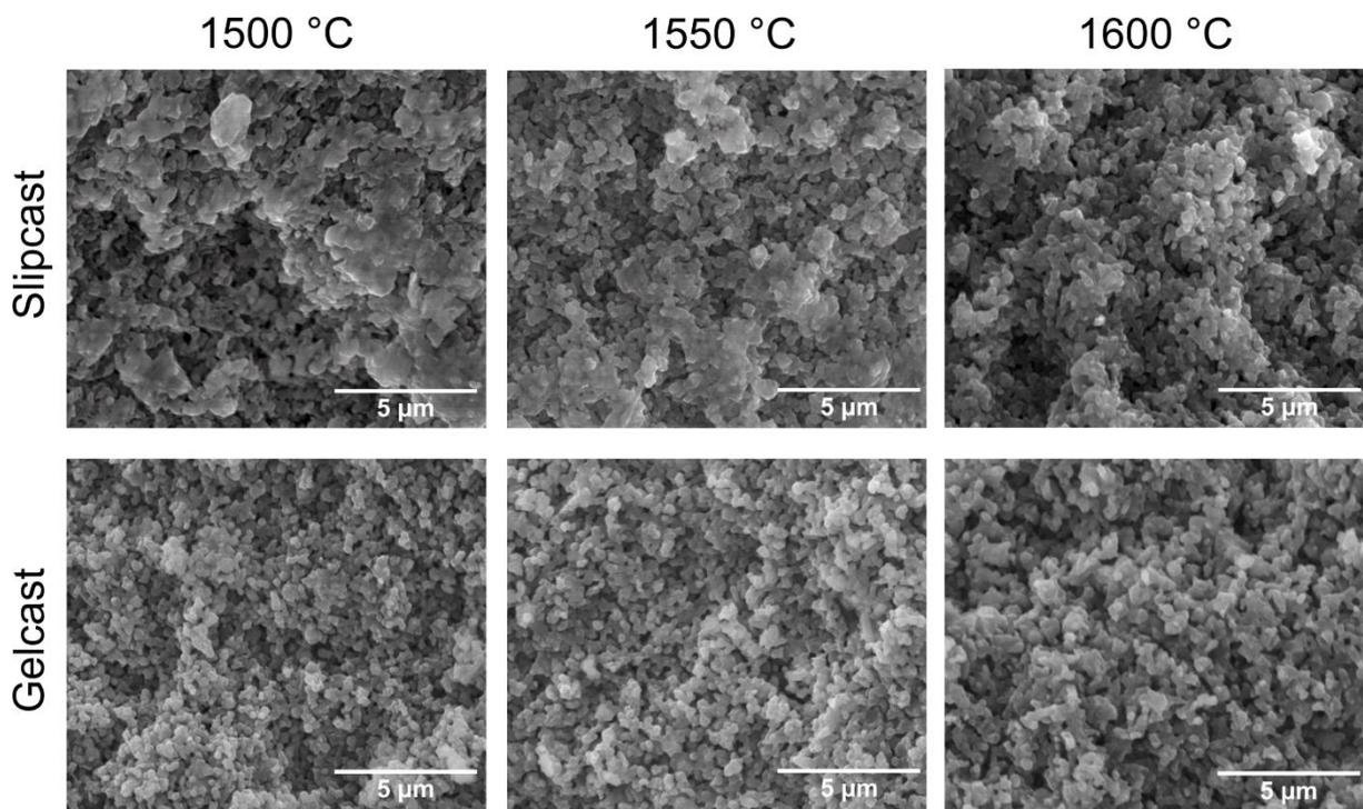
Fig. 2. Fracture surfaces of slip-cast (top) and gelcast samples (bottom), after sintering at various temperatures
