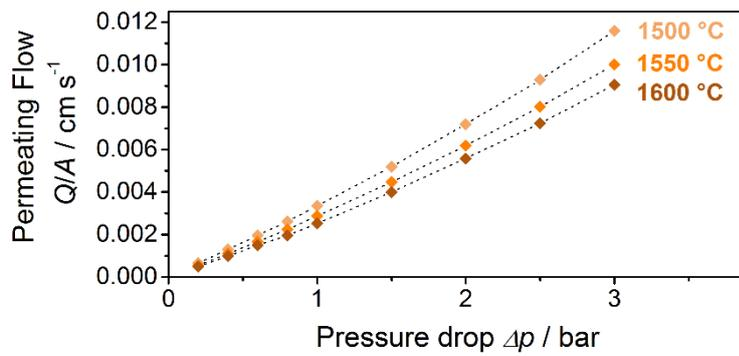
Fig. 4. Typical gas flow curves of samples sintered at different temperatures (exemplary for gelcast materials)
