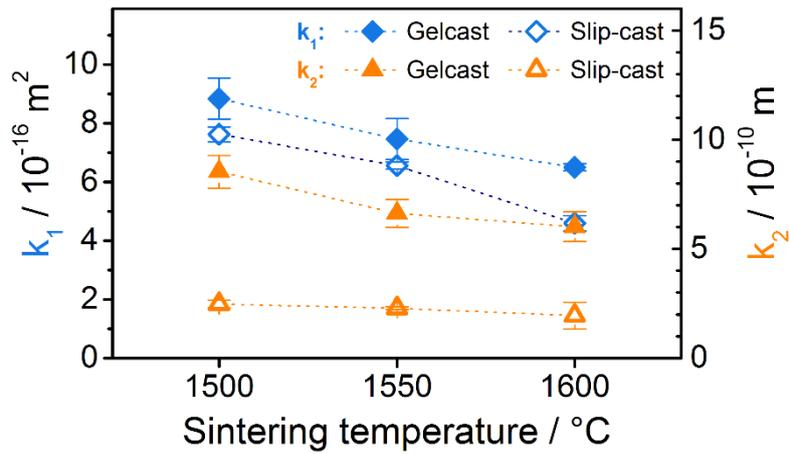
Fig. 5. Effect of sintering temperature on Darcian ( $k_1$ ) and Non-Darcian ( $k_2$ ) permeabilities of slip-cast and gelcast samples
