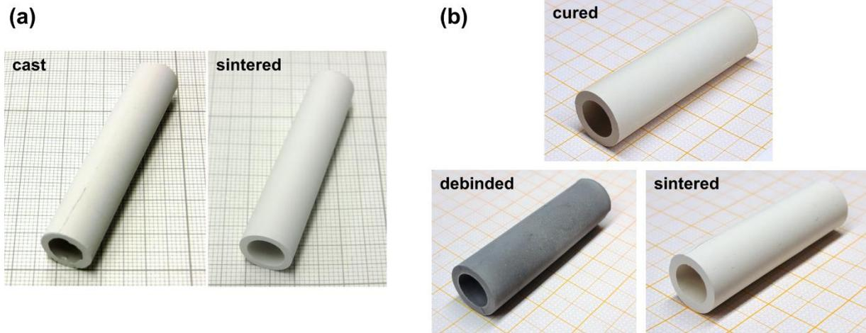
Fig. 1. Morphology and appearance of (a) slip-cast and (b) gelcast silicon nitride specimens during various processing stages
