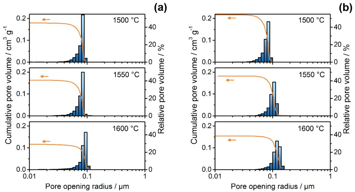
Fig. 3. Pore opening radius distribution of (a) slip-cast and (b) gelcast samples as function of sintering temperature (determined by Hg porosimetry)
