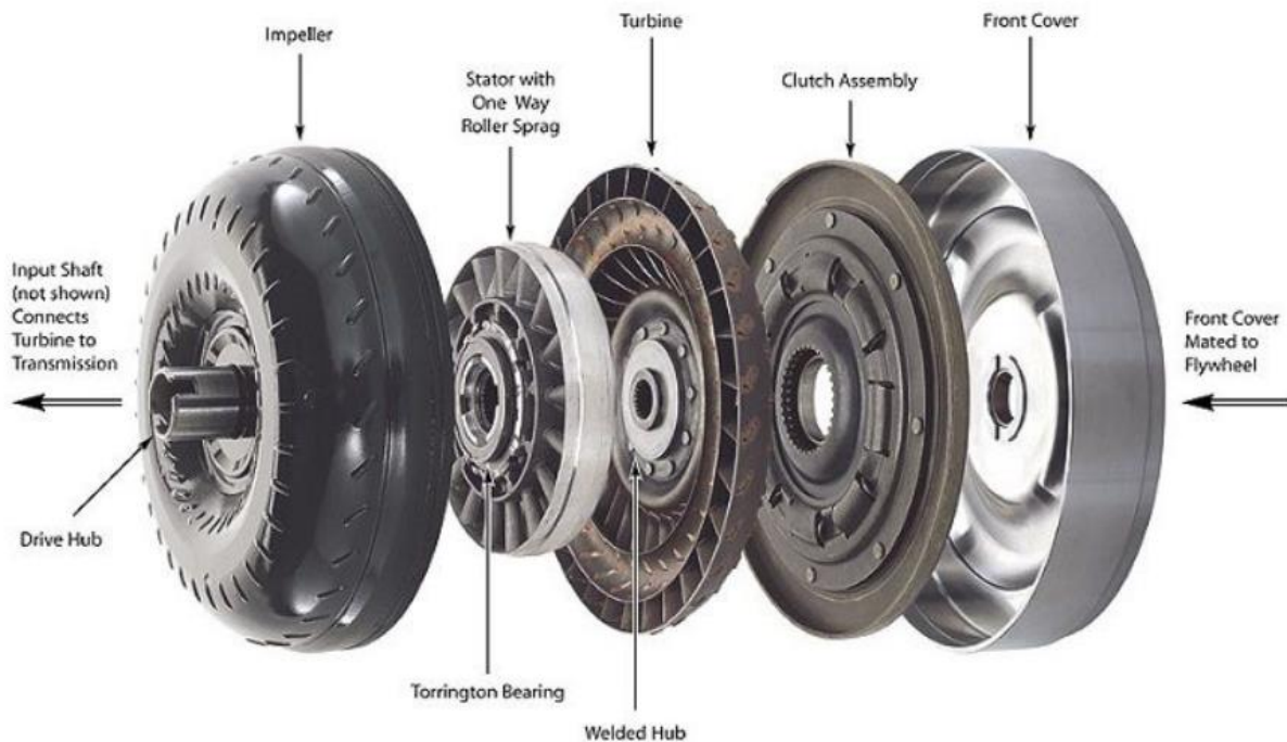
Figure 24: Exploded view automatic transmission torque converter. 151
