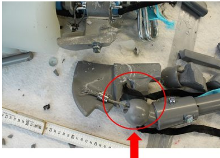
Figure 4.38.: Fracture of the right acetabulum of the Biofidelic Dummy used in crash test wh18.25 (Red circle: Location of fracture; Red arrow: Impact direction)
