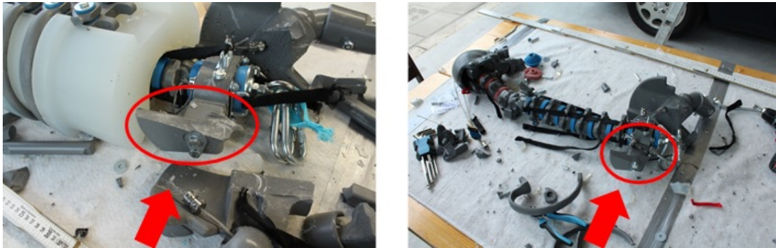
Figure 4.36.: Fracture of the ilium next to the sacroiliac joint of the Biofidelic Dummy (Left: Crash test wh18.25; Right: Crash test wh18.27; Red circle: Location of fracture; Red arrow: Impact direction)
