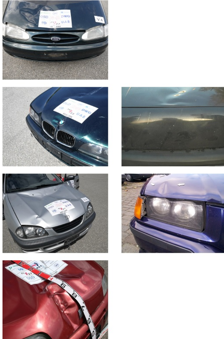
Figure 4.14.: Vehicle damages Žilina Dummy vs. pedestrian. Top left: wh08.27; Upper left: wh08.28; Lower left: wh08.29; Bottom left: wh10.12; Top right: Accident 1; Bottom right: Accident 2
