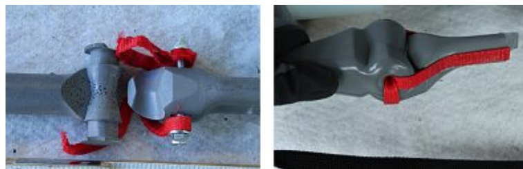
Figure 4.41.: Injuries to the elbows of the biofidelic dummies used in crash tests wh18.22 and wh18.23 (Left: Old design; Right: New design)
