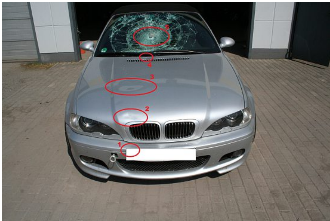
Figure 3.3.: Complete hit. 1: The lower leg impacts the bumper. 2: The upper thigh/hip impacts the bonnet leading edge. 3: The thorax impacts the bonnet. 4: The shoulder impacts the bonnet rear edge. 5: The head impacts the windscreen (DEKRA, n.d.)
