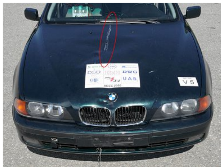
Figure 4.15.: Scratch marks caused by the Žilina Dummy
