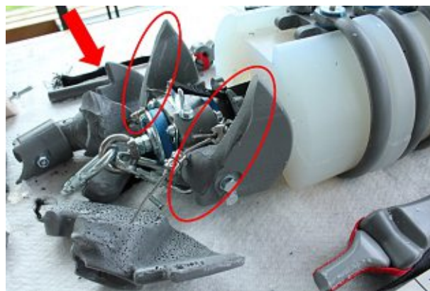
Figure 4.37.: Fracture of the left and right ilium of the Biofidelic Dummy used in crash test wh18.23 (Red circle: Location of fracture; Red arrow: Impact direction)
