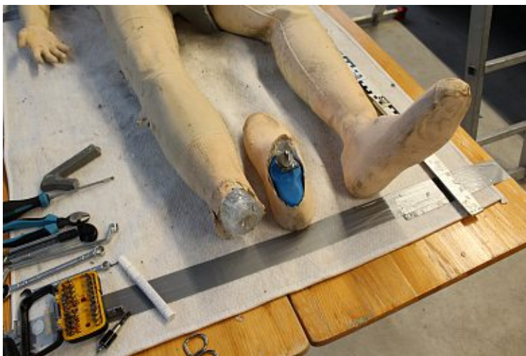
Figure 4.43.: Separation of the right foot of the Biofidelic Dummy used in crash test wh18.27
