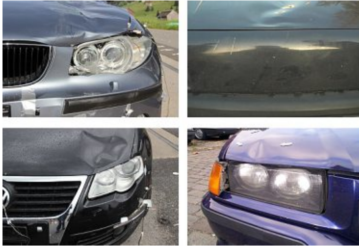
Figure 4.13.: Vehicle damages Biofidelic Dummy vs. pedestrian. Top left: wh18.22; Bottom left: wh18.26; Top right: Accident 1; Bottom right: Accident 2
