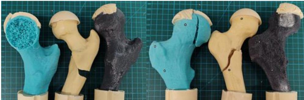
Figure 50: Top: Results of the comparable bones. Bottom: From left to right: SLA printed bone, *ORTHO*bone and *PET* printed bone
