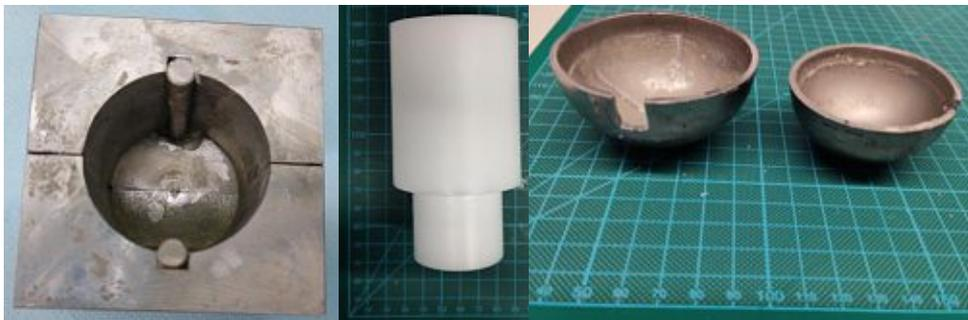
**Figure 28:** Tool for embedding of the shaft on the left and turned fixture and the cups for the embedding of the head on the right.
