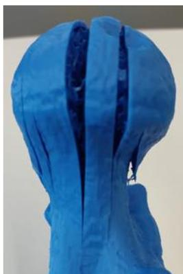
**Figure 42: Splitting of the test bone with a non-embedded head.**
