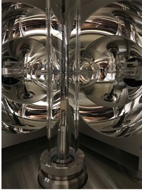
Figure 3: Optical floating zone furnace with sample rods.
