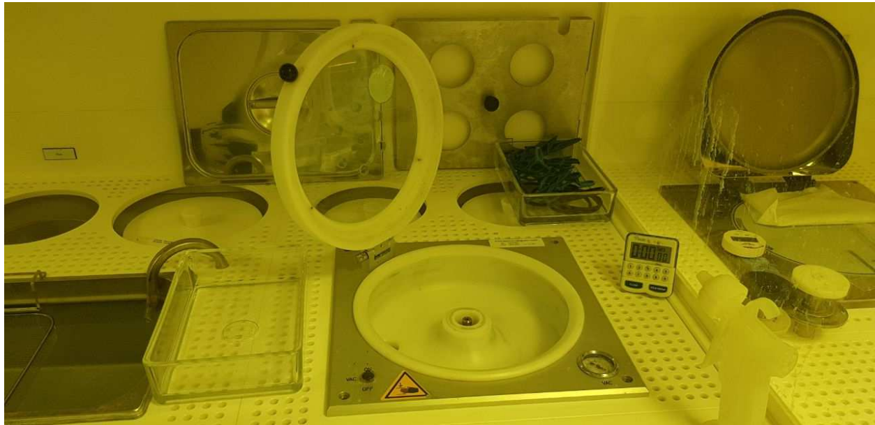
Fig.3.21. Spin- coating printer SPIN150i
