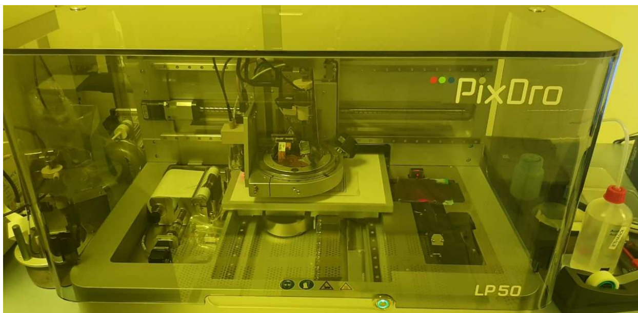
Fig.3.20. Inkjet printer, PixDro-LP50 with a print head; Dimatix Spectra
