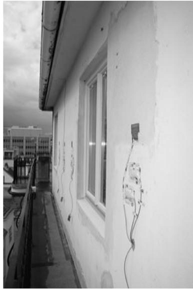
Figure 2.13 View of installed sensors on the existing wall; temperature and humidity sensors as well as the heat flow plates of the test areas on the south façade (source: Schuss et al. 2017)
