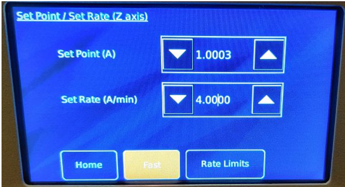
Figure A.11: Subpanel of MercuryIPS that displays the current set point and the ramp rate.
