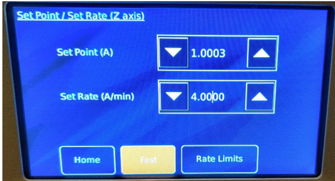
Figure A.19: Subpanel of MercuryiPS that displays the current set point and the ramp rate.
