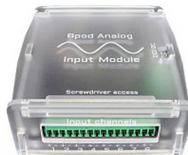
Figure 5.8: Bpod analog input module image from Sanworks (Sanworks 2021)
