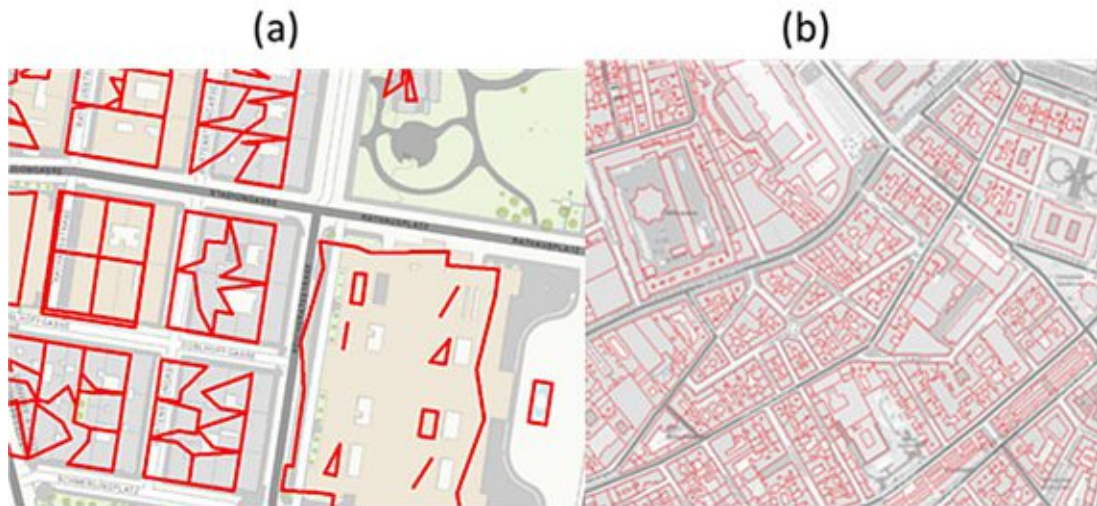
Figure 46: Sampling errors when importing building outline polygons at (a) 20m and (b) 0.3m resolution
