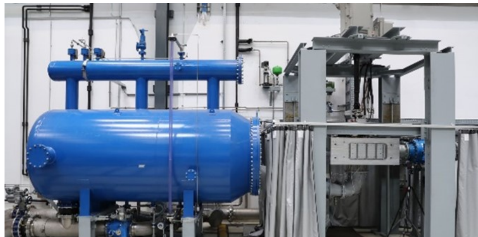
Figure 6. Test rig with scale reduced model of a radial pump turbine at the hydraulic lab of the Institute of Energy Systems and Thermodynamics, TU Wien.
