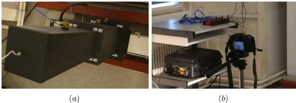
Fig. 4.6: Data monitoring system: (a) attached accelerometers at the back of the test specimens; (b) wireless monitoring system and camera for documentation
