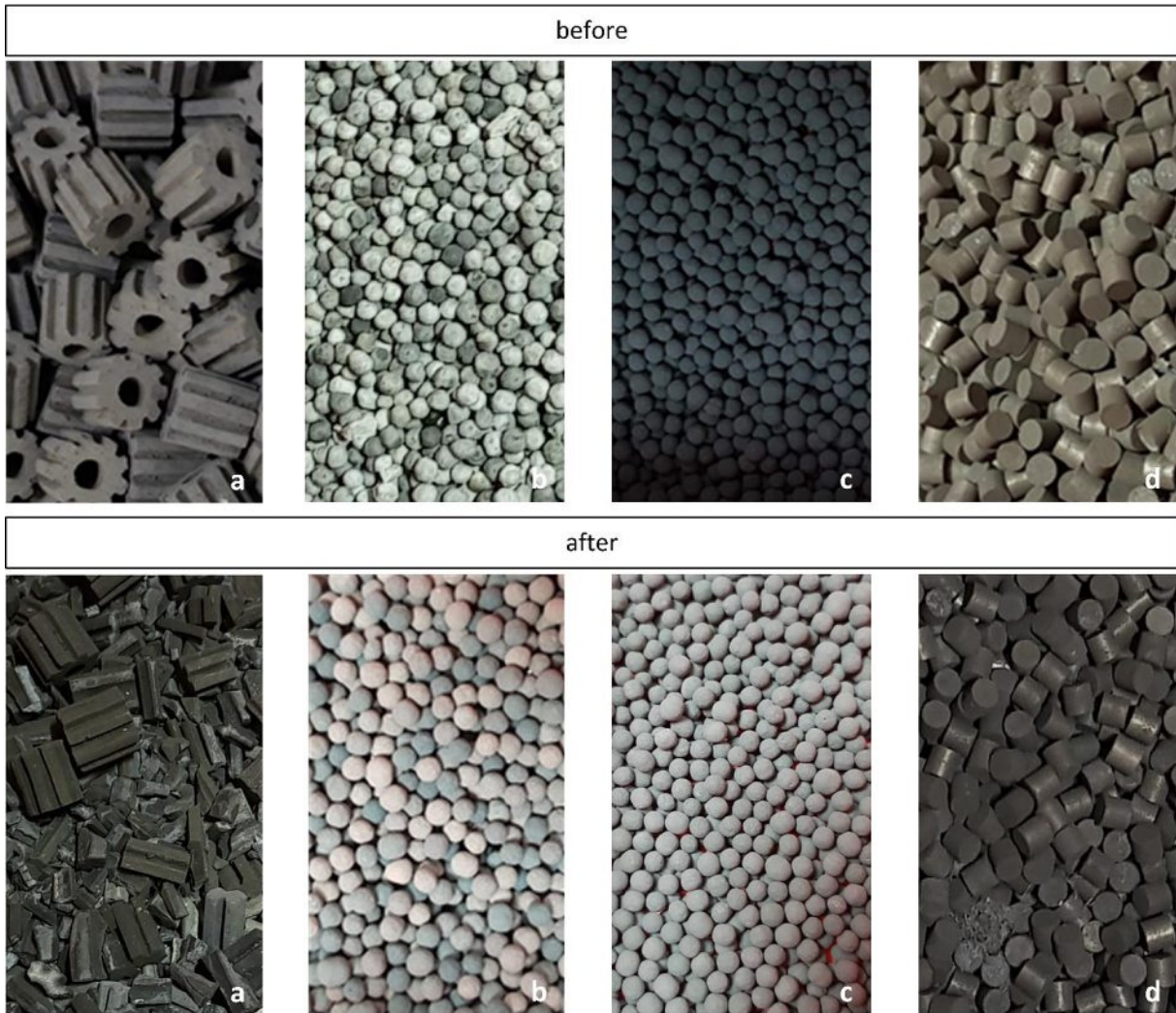
figure 43: Catalysts Before and After – In this image a real size picture of the catalysts, CAT 1 (a), CAT 2 (b), CAT 3 (c) and CAT 4 (d) is shown before and after the test were carried out. Catalyst (a) needed to get crushed before it was possible to fill it into the reformer.
