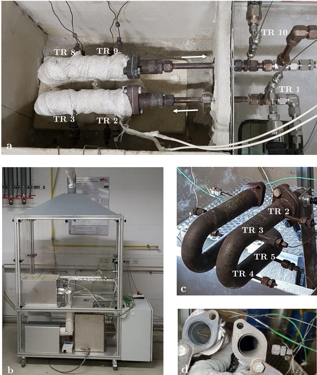
Figure 9: Test Stand – Image (a) shows the reformer and how it was integrated into the test facility. During the measurements, the box around the reformer, was filled with a thermo granulate for a better insulation. The flow direction is indicated by white arrows. Image (b) shows the whole test stand. Image (c) shows the reformer without any insulation. Image (d) shows the position of the thermocouples inside the empty reformer before it was filled with a catalyst material.
