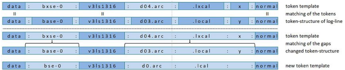
Figure 5.7: Token_char algorithm matching. Dark blue parts represent token-structures and light blue parts character-structures. Colons represent any fixed set of predefined delimiters [WHL + 20].
