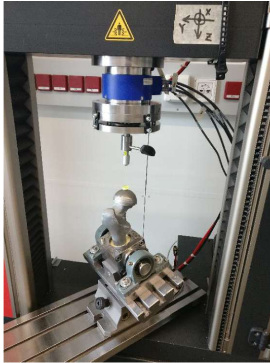
Figure 30: Laser Alignment of the Caput femoris for the right position for compression test
