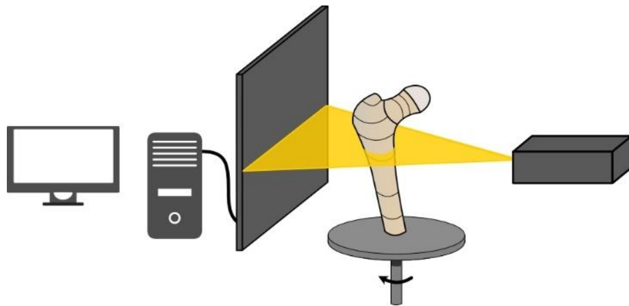
Figure 11: schematic principle of \mu -CT measurement
