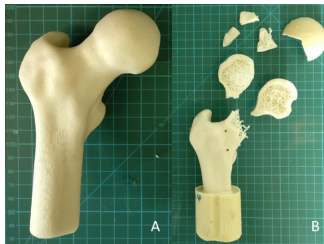
Figure 43: Printed OB sample (A) before (B) after compression test
