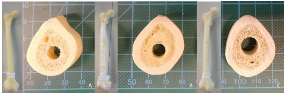
Figure 5: PU based Bones. (A) ORTHObones Standard Femur, right (3B Scientific GmbH, 20459 Hamburg Germany) (B) ORTHObones Premium Right Femur (3B Scientific GmbH, 20459 Hamburg Germany) (C) Right Femur with distal canal opening (SYNBONE AG, 7205 Zizers, Switzerland)
