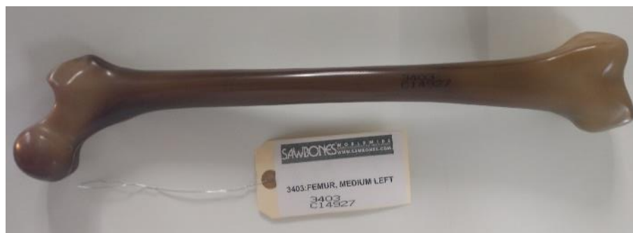
Figure 4: SGFR Composite Bone. Femur, 4th Gen., Composite, 17 PCF Solid Foam Core, Medium (A Pacific Research Company, Vashon Island, Washington 98070, USA.)
