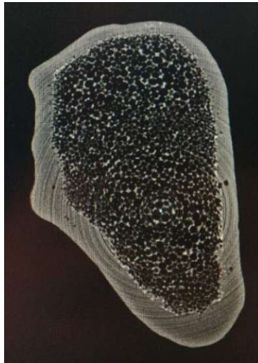
Figure 13: Ring Artefacts shown on the basis of a reconstructed \mu -CT scan of a purchased artificial bone
