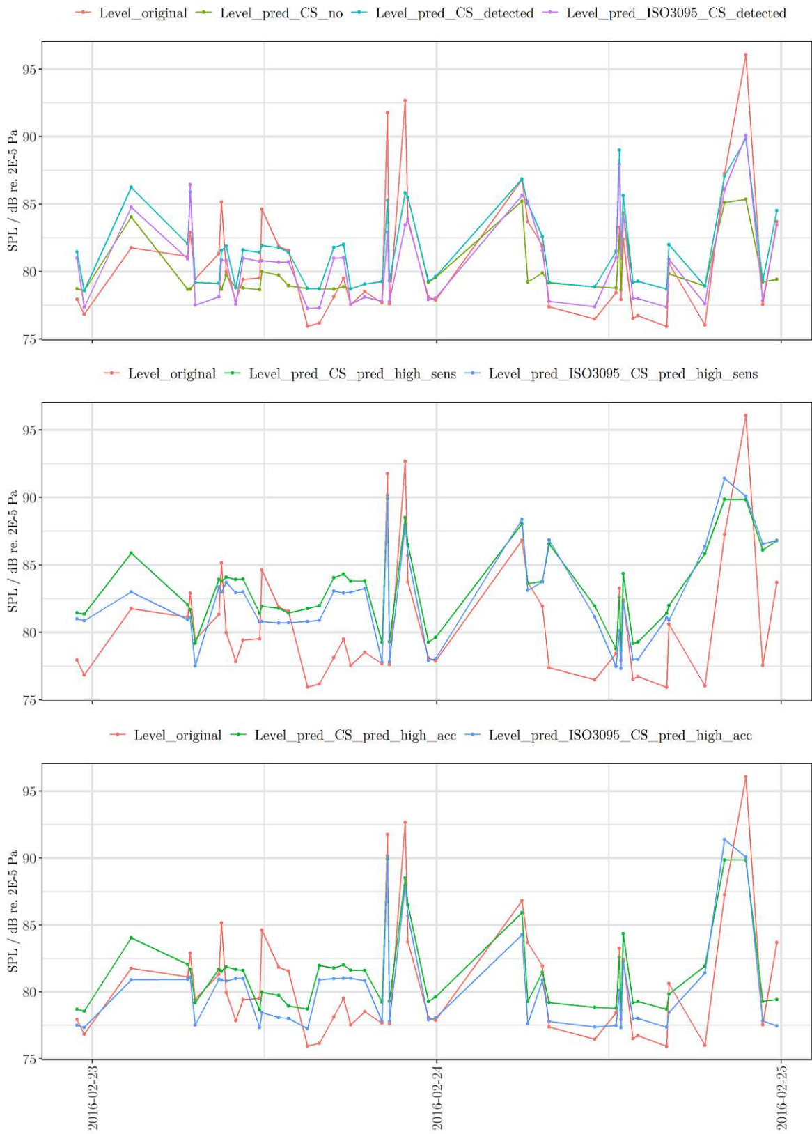
Figure 90: Exemplary time series plots depicting two days of originally measured equivalent continuous noise levels versus different prediction outcomes in C4
