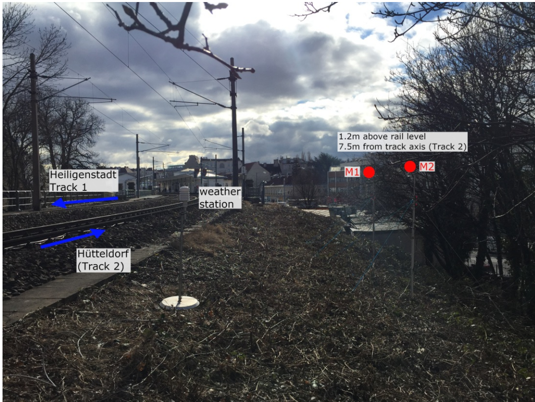
Figure 17: Overview of the measurement section of C4 (© psiacoustic Umweltforschung und Engineering GmbH)
