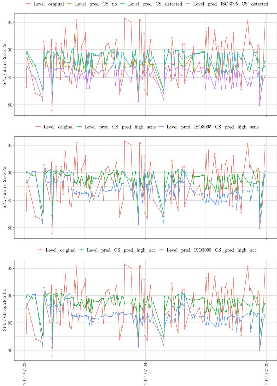
Figure 88: Exemplary time series plots depicting two days of originally measured equivalent continuous noise levels versus different prediction outcomes in C2
