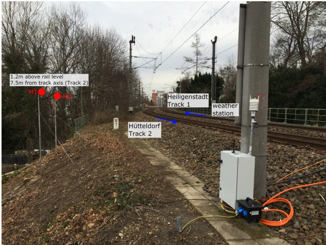
Figure 21: Overview of the measurement section of C5 (© psiacoustic Umweltforschung und Engineering GmbH)
