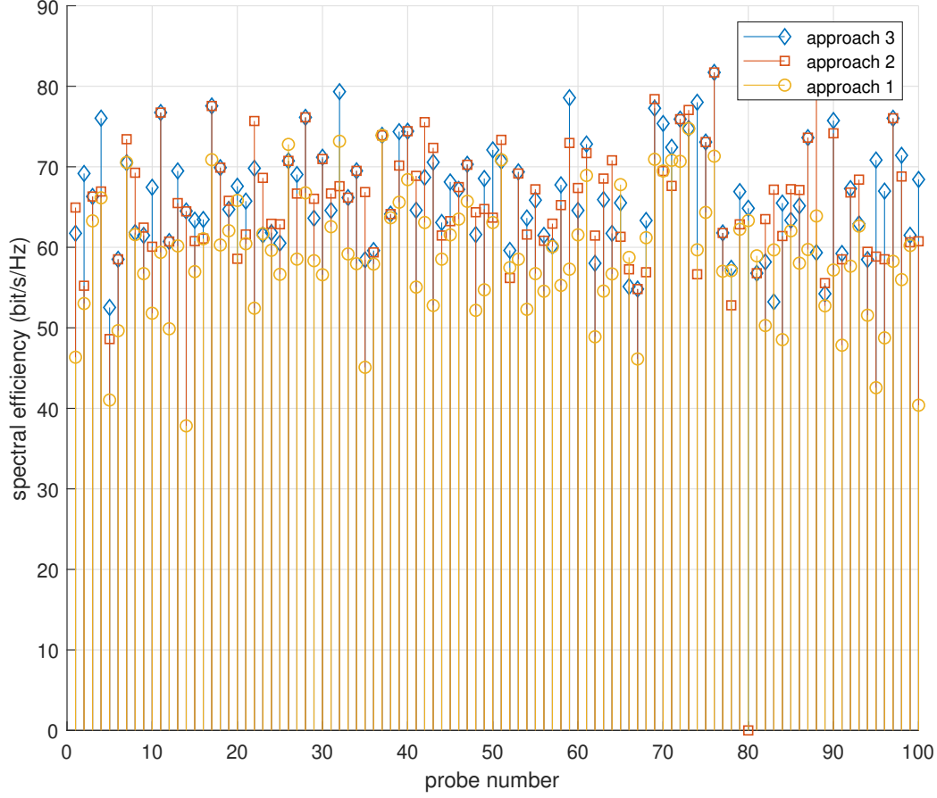
Figure 7.14: Comparison of the spectral efficiency achieved by the proposed decentralized scheduling schemes.
