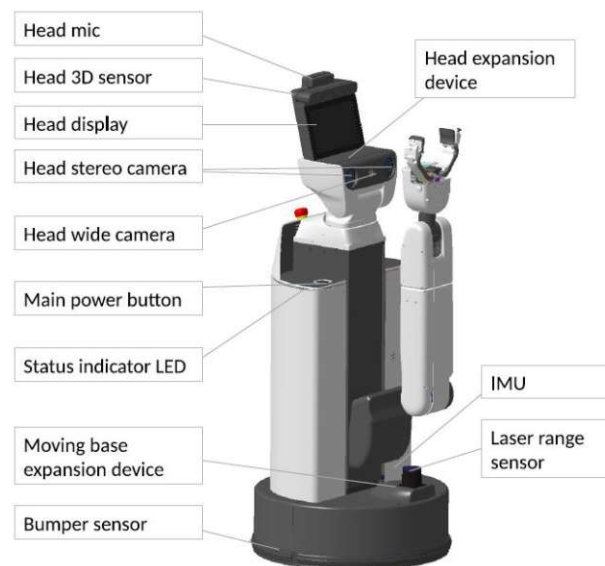
Figure 2.3: The HSR is equipped with various sensors [12]
