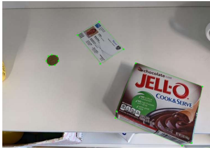
Figure 4.2: A training image with the three object classes: card, box and coin
