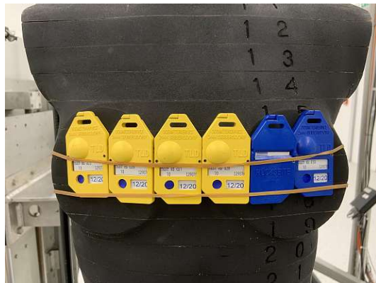
Figure 3.9: Four TLD attached on the ISO slab (left). TLD attached on the Alderson phantom (right). The result for the switched TLD served as additional information for the impact of carrying a TLD improperly and was not included into the calculations presented in this section.
