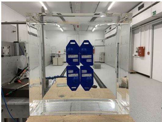
Figure 3.9: Four TLD attached on the ISO slab (left). TLD attached on the Alderson phantom (right). The result for the switched TLD served as additional information for the impact of carrying a TLD improperly and was not included into the calculations presented in this section.
