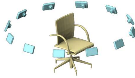
Figure 4.5: Camera placement for the MVCNN dataset generation [12]
