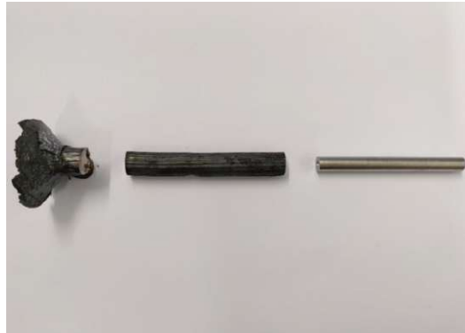
Fig. 6: Binder material after extrusion with and without steel coat
