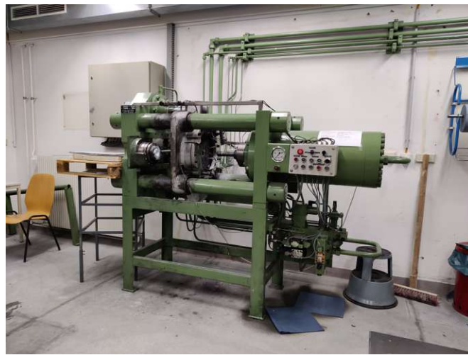
Fig. 5: Hot extrusion press at TU Wien
