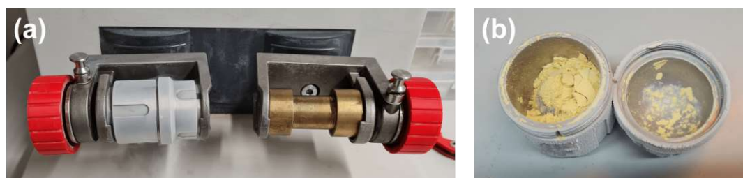
Figure 4.3: (a) Swing mill (MM400, RETSCH) with a steel container, containing pollen, left and a counter weight right. (b) Pollen after milling in the steel container.
