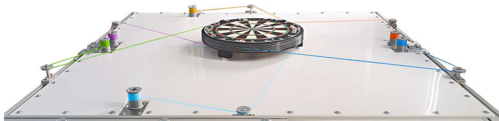
Figure 8.4: Guiding surface. The white cables are colored for better visibility.
