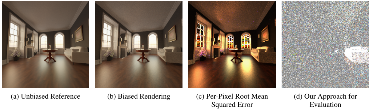
Figure 1: Here, we illustrate the potential of our proposed approach for the evaluation of Monte Carlo (MC) rendering techniques. It is based on the sampling distribution of the mean (SDM). Image (a) shows a reference rendering and (b) an artificially biased rendering for which the reflectance of the couch on the right-hand side was reduced. Our approach (d) can reveal differences between both renderings that are difficult to identify through visual comparison or other metrics, e.g., the (normalized) root mean squared error (RMSE) calculated for each pixel (c). This circumstance suggests the viability of using SDM-based approaches for the per-pixel comparison of MC renderings.
