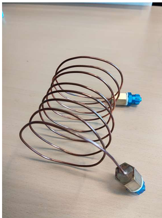
Figure 6.1: Copper tube functioning as RF coil. Its outside diameter is 2 mm and the inside diameter 1 mm. Adapters for the water cooling circuit are welded onto the ends of the coil and are applicable for tubes with an outside diameter of 8 mm and an inside diameter of 5 mm. Connections for the electrical circuit have not yet been implemented.
