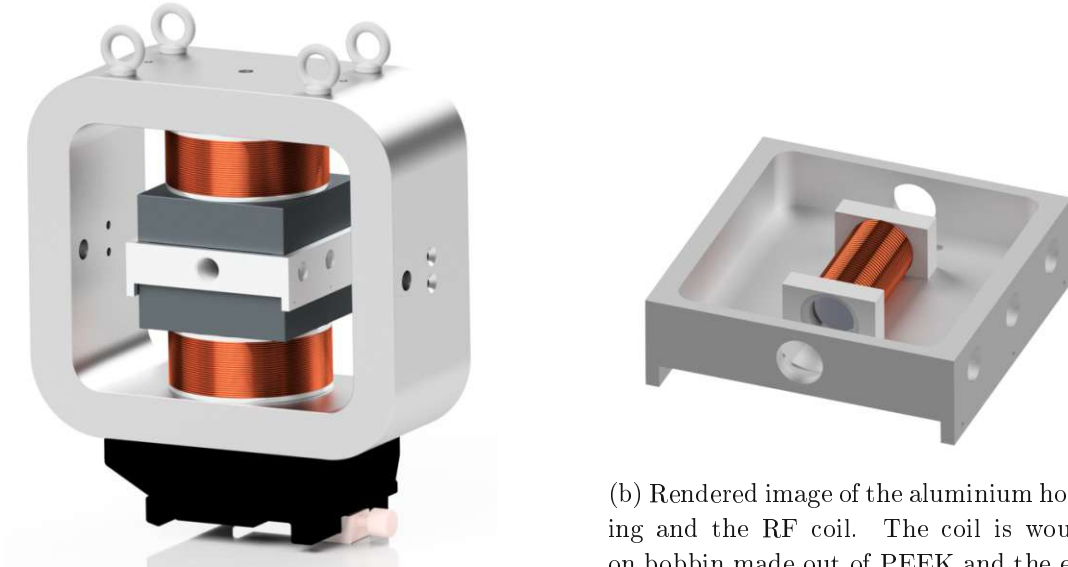
(a) Rendered image of the RF flipper used for the spin chopping system. The B_0 field is produced by a copper coil with iron core. The aluminium box in between the iron pole shoes is shown in figure (4.3b).
