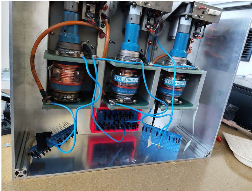
Figure 5.9: Photo of the capacitors inside the aluminium box, which prevents the RF radiation to disturb the detector's amplifier electronics.
