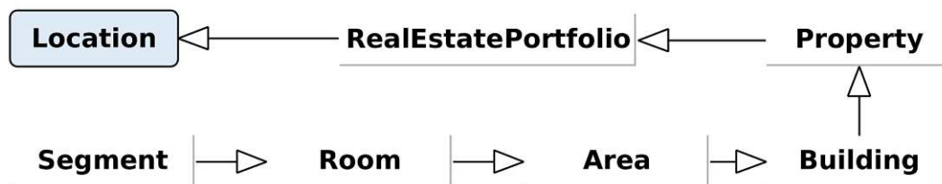
Figure 3.11: Location class hierarchy according to the multilayer-model presented in part 1 of the VDI 3814 guideline [26]
