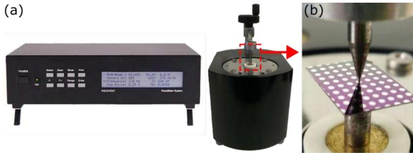
Figure 9: (a) Optical photograph of a piezometer PM300 from Piezotest Ltd. and (b) a sample with a piezoelectric thin film and several aluminum pads, clamped between the electrodes of the piezometer.
