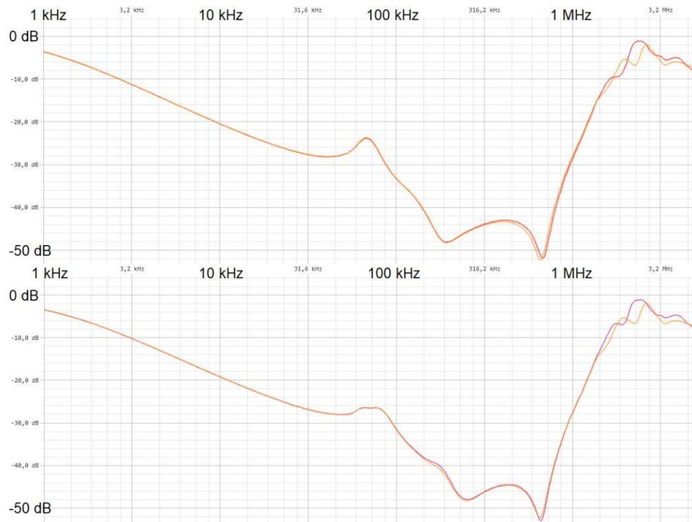
Figure 4.1: Stator 1 , Phase U : The upper plot shows the fault-free case, the lower plot an inter-turn fault between access point C and D (i.e. a single turn is short-circuited, table 4.1). In both figures, the red curve represents the test with U1 as input terminal. The orange one was recorded with U2 as input terminal.
