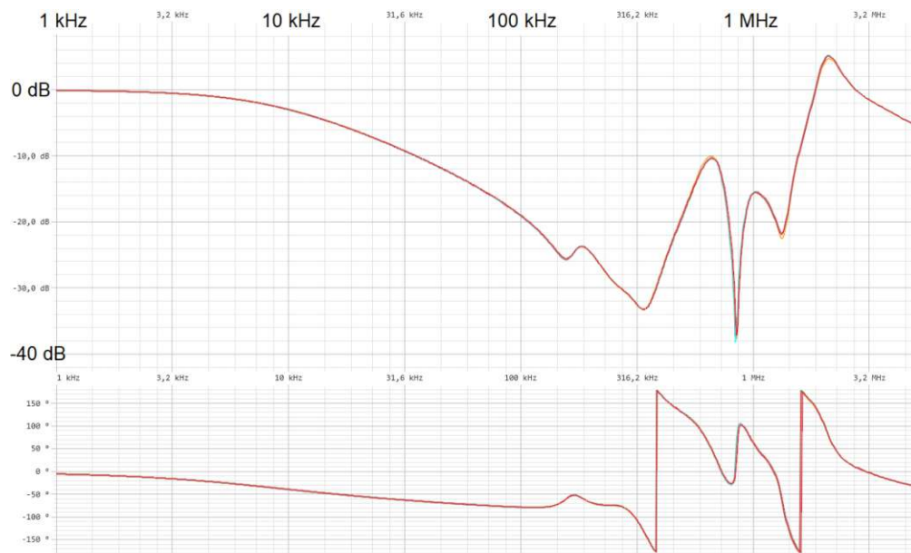
Figure 4.4: Stator 2 , Phase U , single inter-turn faults: E-F (orange), G-H (purple), D-E (turquoise) and C-D (red).
