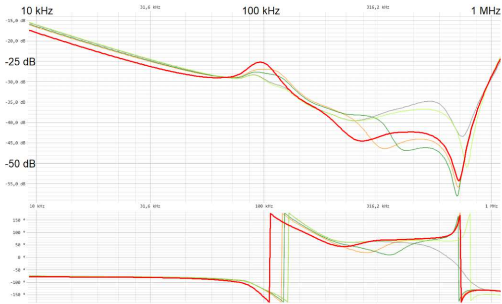
Figure 4.12: Fingerprint measurement (phase U ) of stator 3 : healthy fingerprint (red, thick), E-F (1 turn, orange), D-F (2 turns, dark green), A-F (16 turns, grey) and A-G (27 turns, light green).
