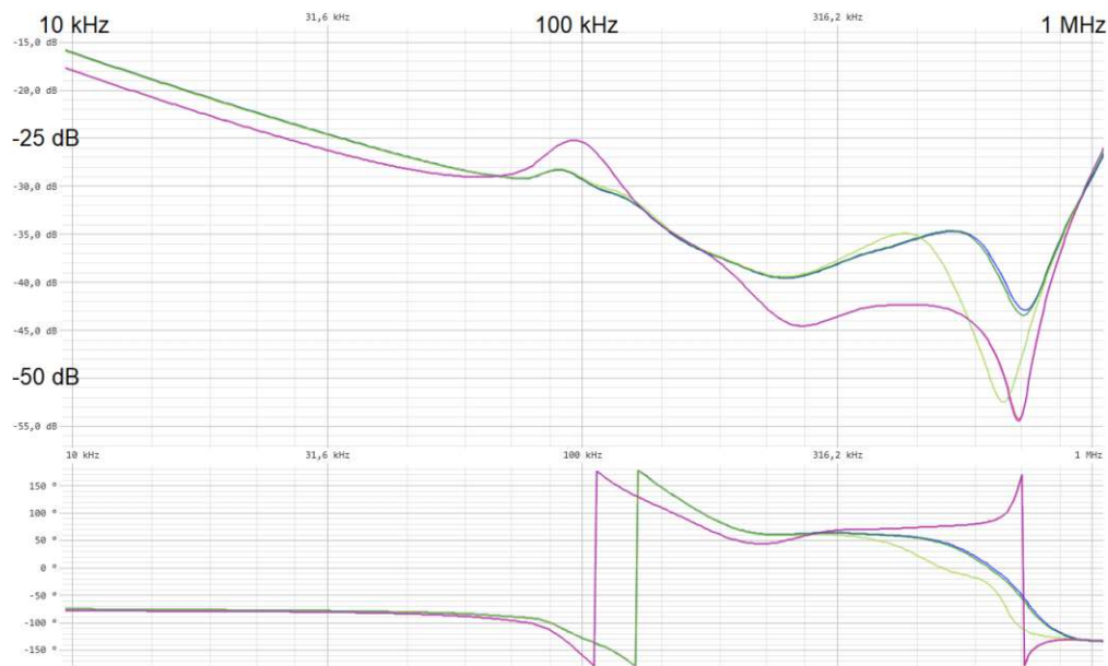
Figure 4.23: Stator 3: The symmetric case A-K (purple) is identical to the fingerprint U (red). It is interesting that E-K (asymmetric by 15 turns, dark green) is nearly undistinguishable from the inter-turn fault A-E (15 turns, blue). Fault C-K (asymmetric by 7 turns) is also similar to A-E over a wide frequency range. All asymmetric faults fulfill the amplitude gap and resonance shift fault condition, therefore, the malfunction can be identified.
