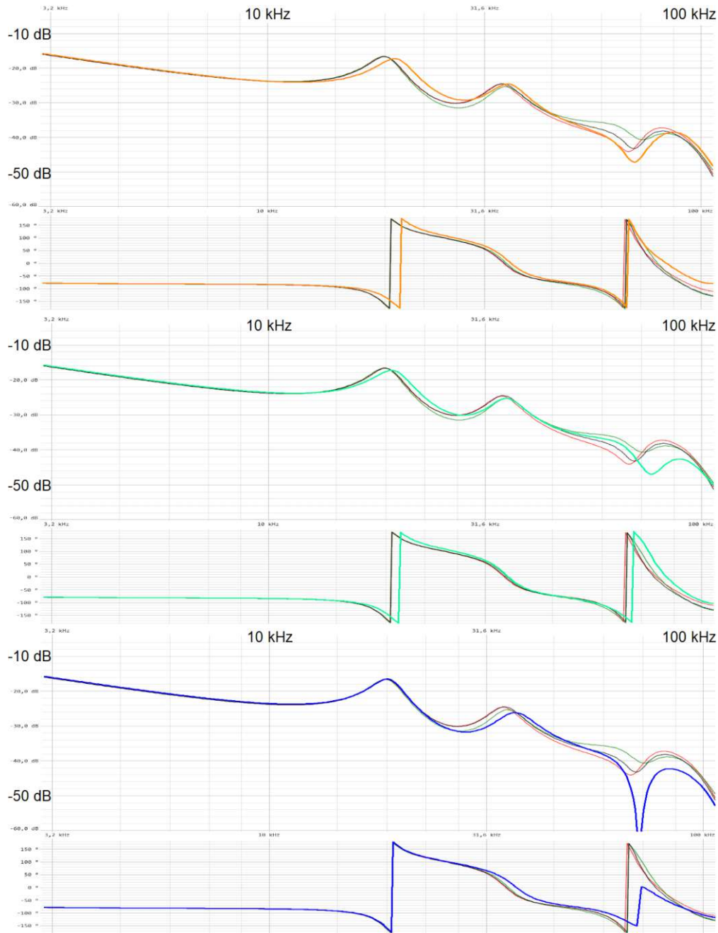
Figure 4.29: Extended winding measurement of stator 1 : phase 1 (red), phase 2 (green) and phase 3 (black), compared to the single inter-turn fault D-E implemented in phase 1 (upper figure, fault at the beginning), phase 2 (middle figure, fault at the end) and phase 3 (lower figure, fault in the middle). For a better visualization, the figures are squeezed so that all images are one underneath the other on one side.
