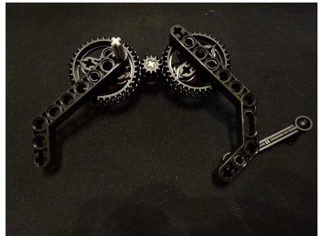
Figure 34: Legs and gears used for the locomotion system in figure 33
