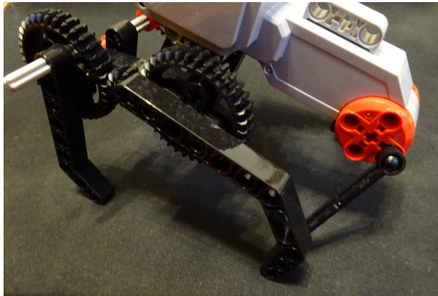
Figure 33: FOOTSTEP locomotion system
