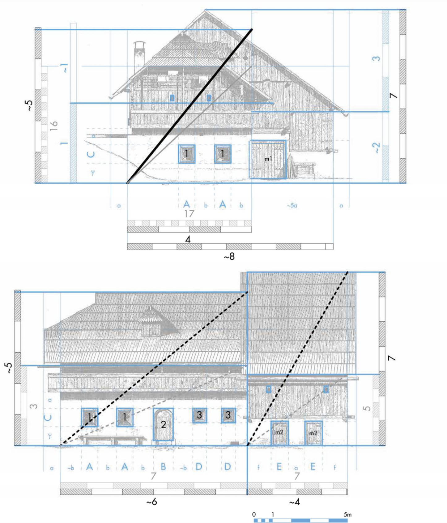
Fig. V.45 Geometrical analysis of front elevation: (C02) "Unterdebernigg-Keusche", House No. 14 in Pöckau near Arnoldstein in Gailthale Fig. V.46 Geometrical analysis of side elevation: (C02) "Unterdebernigg-Keusche", House No. 14 in Pöckau near Arnoldstein in Gailthale
