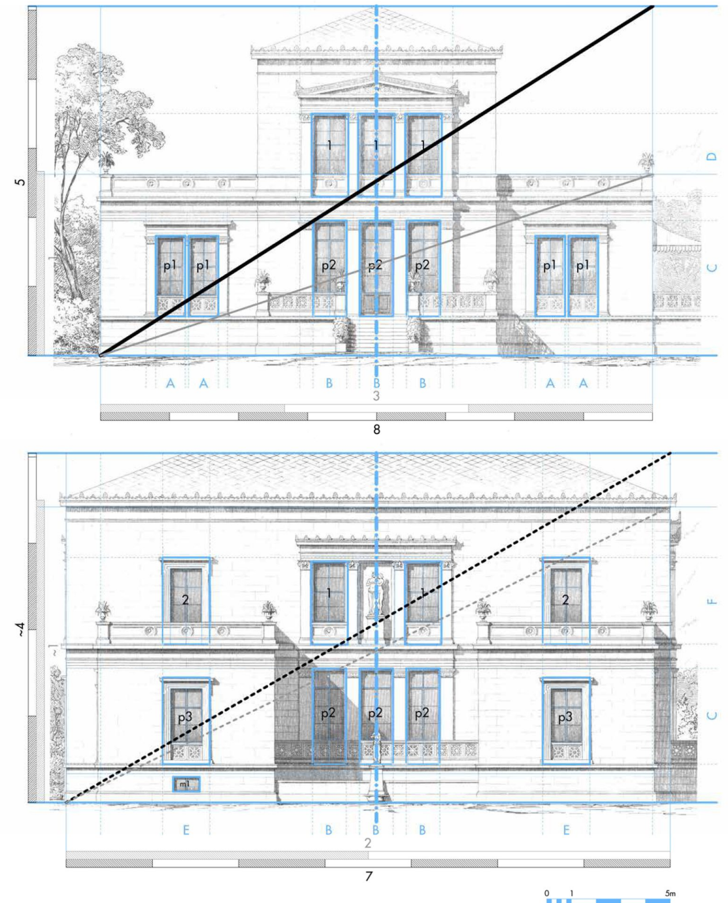
Fig. P.70 Geometrical analysis of front elevation: (U02) Summerhouse, Baden near Vienna Fig. P.71 Geometrical analysis of side elevation: (U02) Summerhouse, Baden near Vienna
