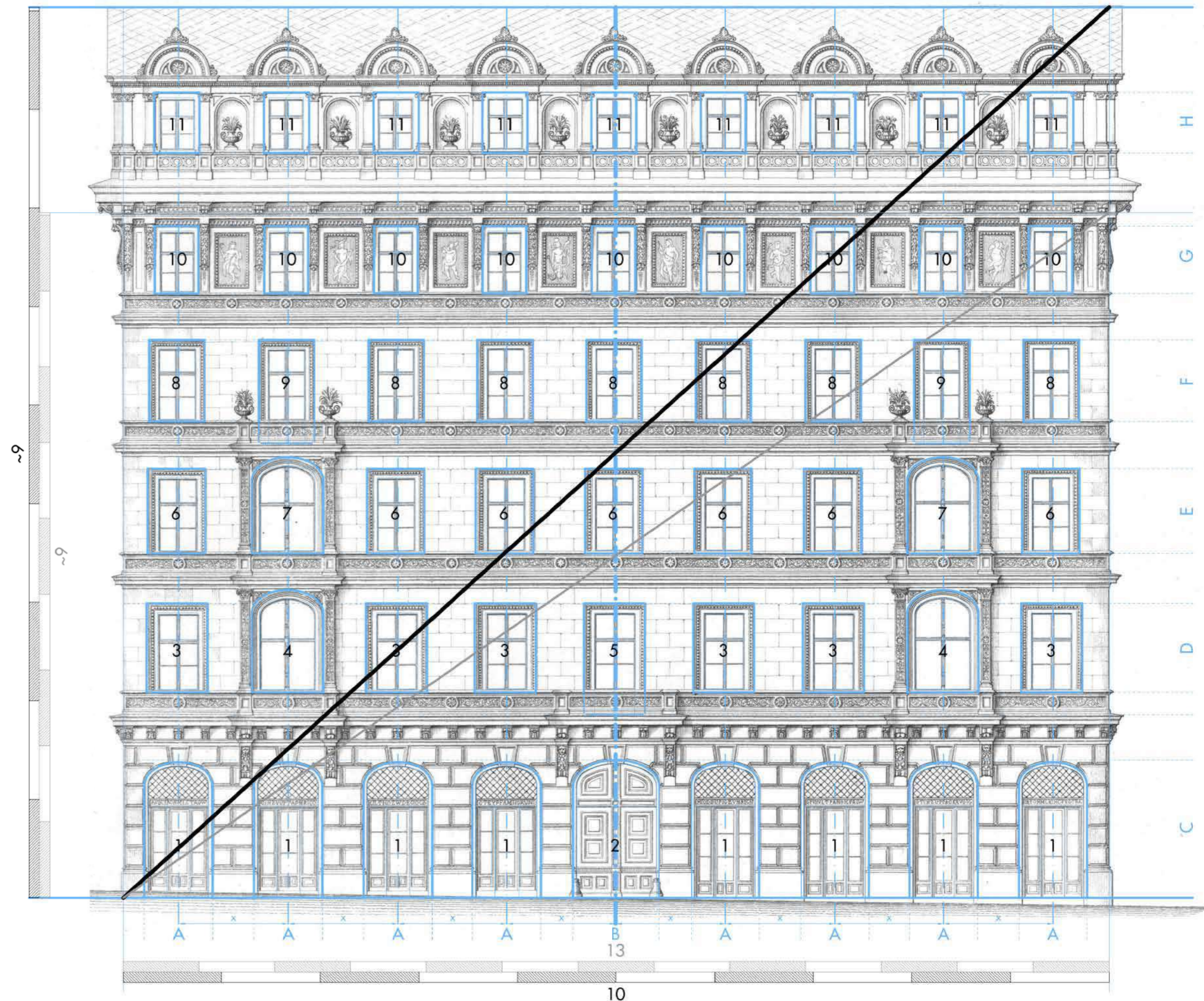
Fig. P.179 Geometrical analysis of front elevation: (VieR09) Residential house of Mr. Alexander Ritter von Schöllner, Ring Road, Opening 6
