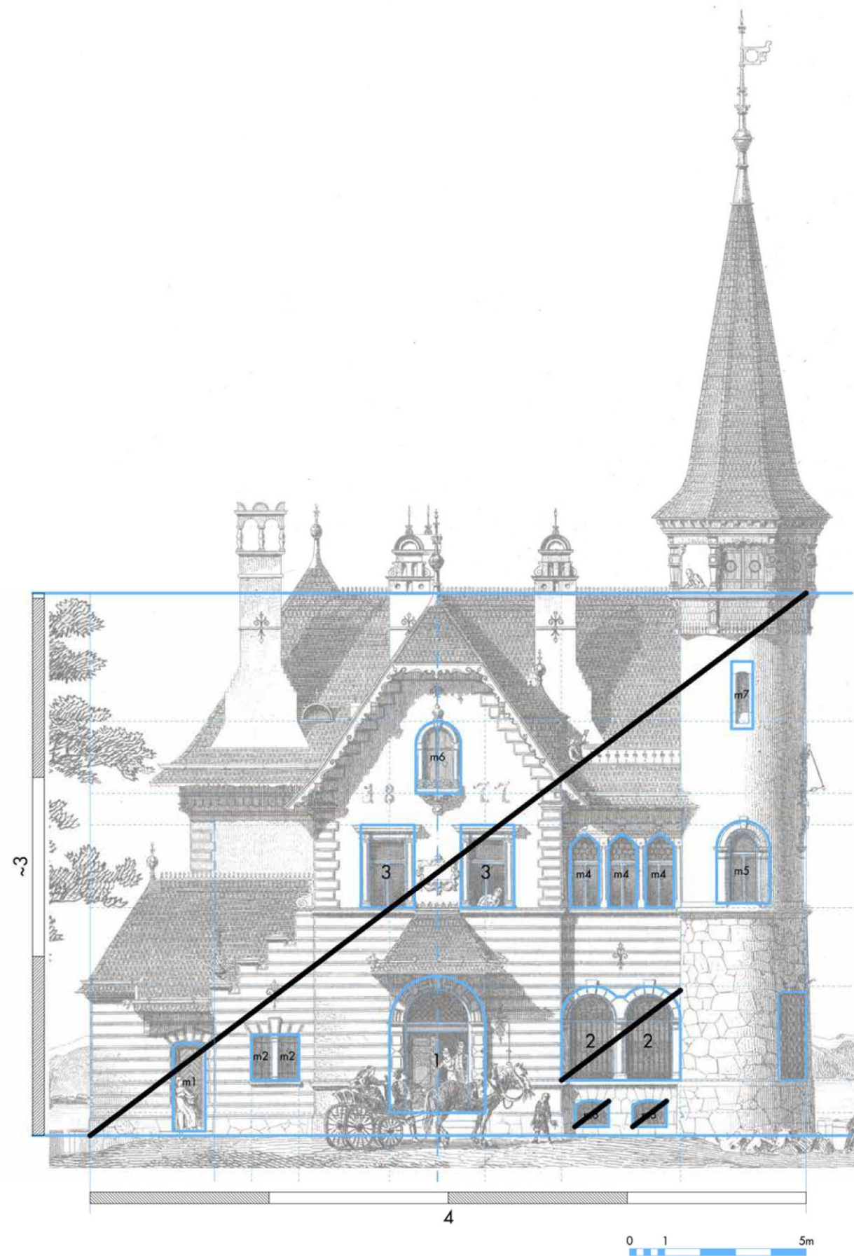
Fig. P.59 Geometrical analysis of front elevation: (U04) Villa Paulick, Seewalchen am Attersee
