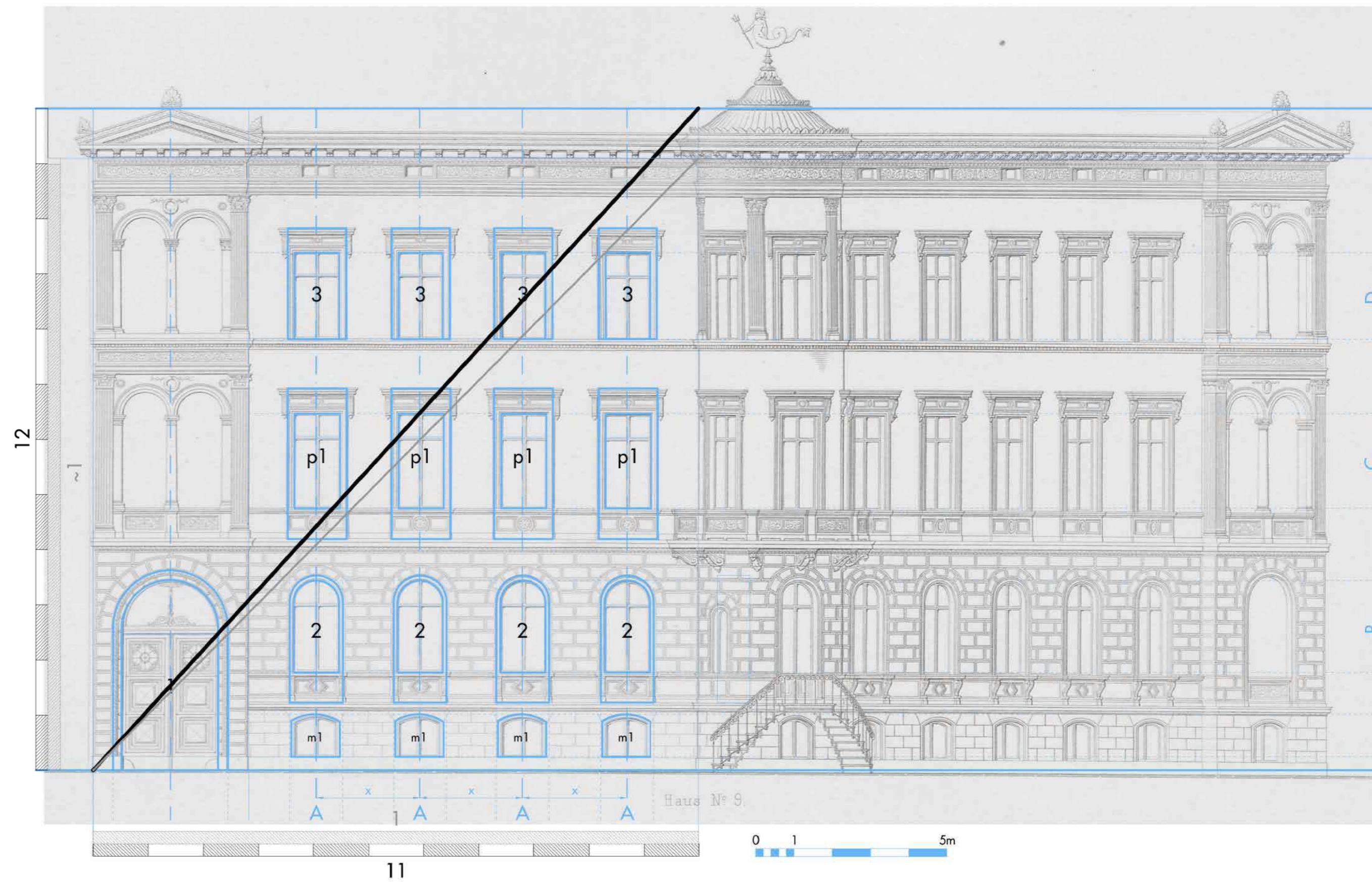
Fig. P.114 Geometrical analysis of front elevation: (BerV08) Residential house No. 9, Victoria-Straße
