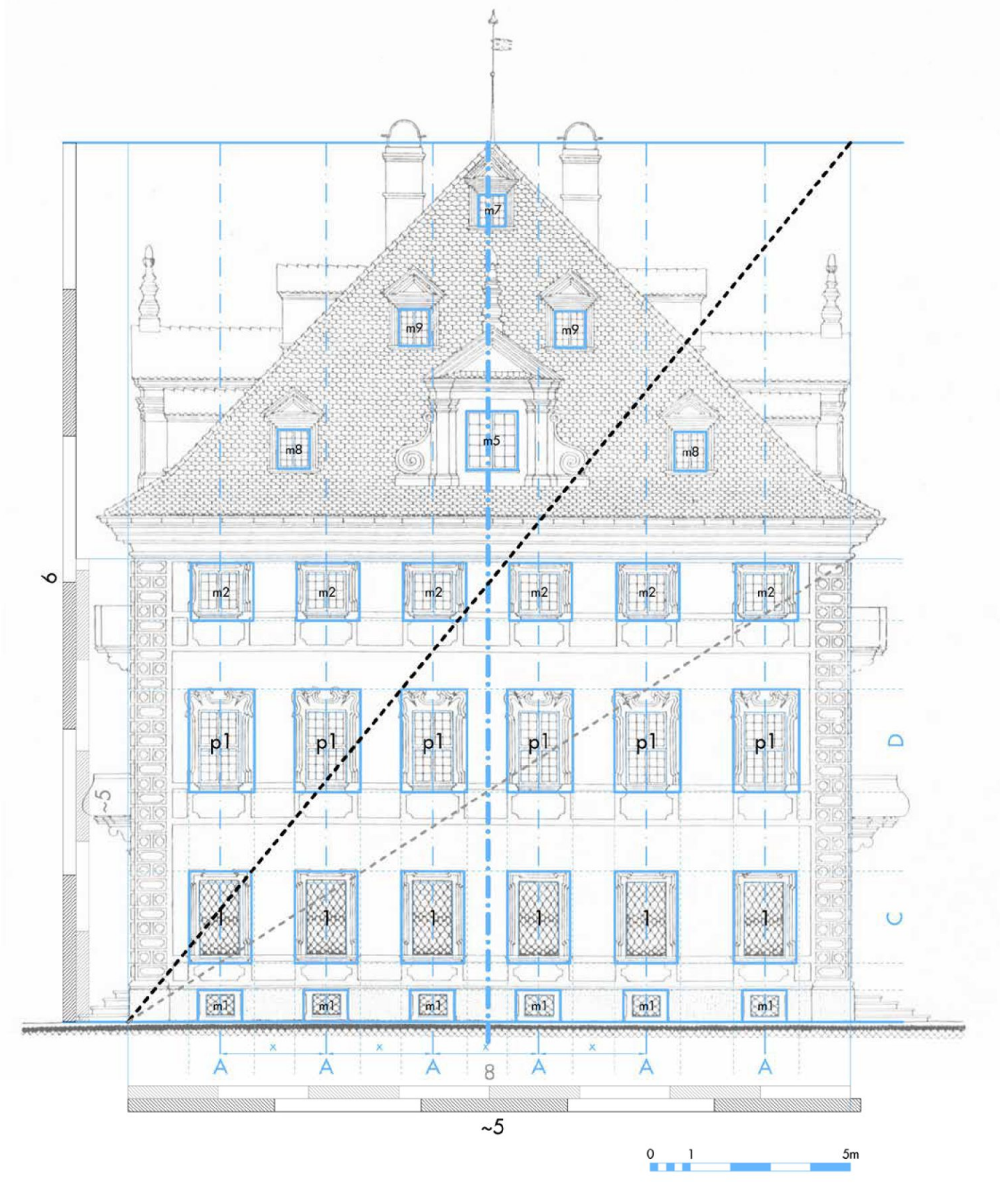
Fig. P.37 Geometrical analysis of side elevation: (G01) Palais Donatz, Sils im Domleschg
