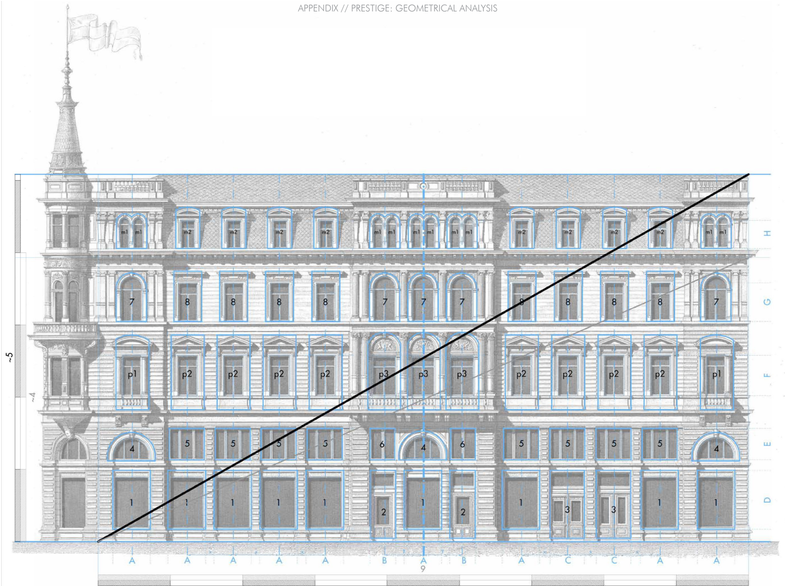
Fig. P.79 Geometrical analysis of front elevation: (Ba-Wü01) Residential house of Mr. K. Model, Karlsruhe in Baden
