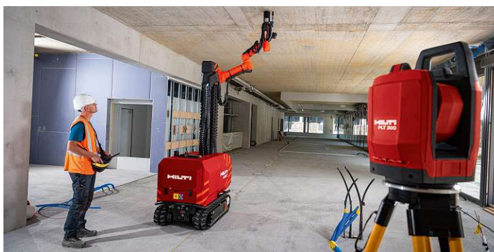
Abb. 3.30: Bohrroboter Hilti Jaibot [179]
