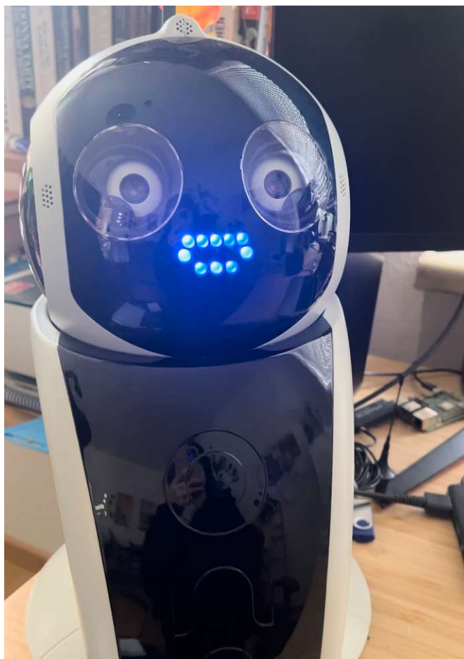
Figure 3.2: QBo robot when talking to the user. The nose LED is turned off and the mouth LEDs are mimicking movement of the mouth when speaking.
