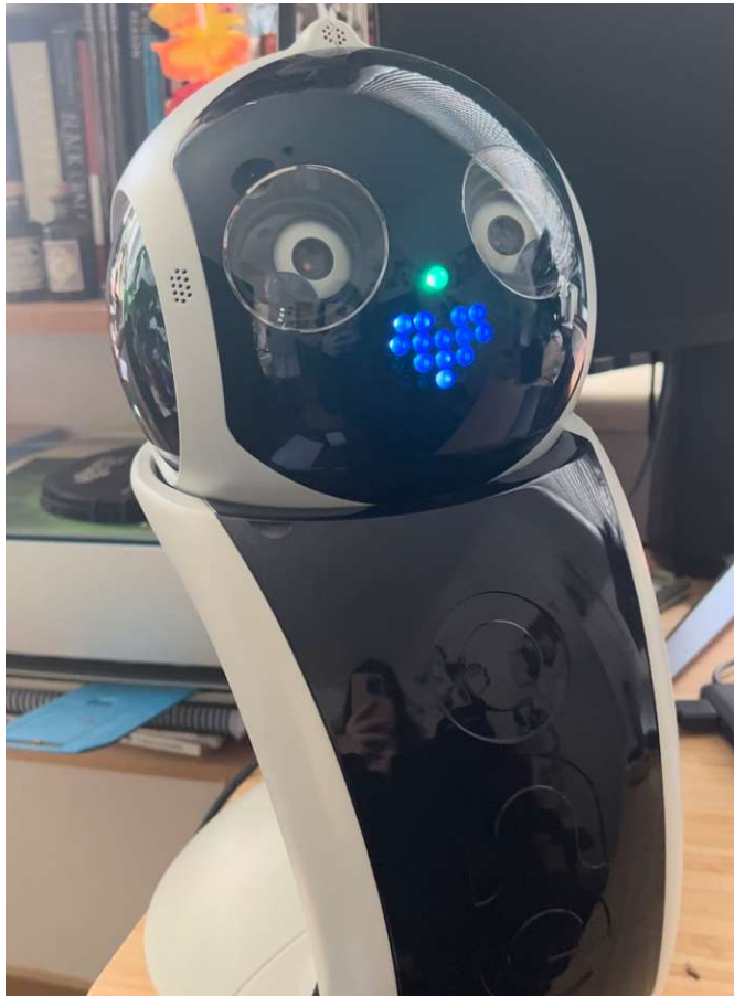
Figure 3.3: QBo robot when listening to the user’s input. The nose is green, indicating waiting and the mouth is in the default position.
