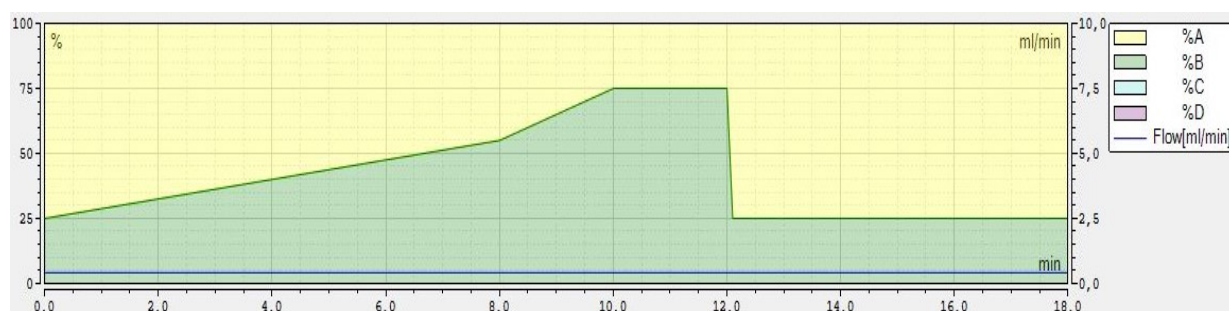
Figure 2.5: Mobile phase concentration profile over time with A - type-1 purified water and B - AcN, both containing 0.1 % TFA
