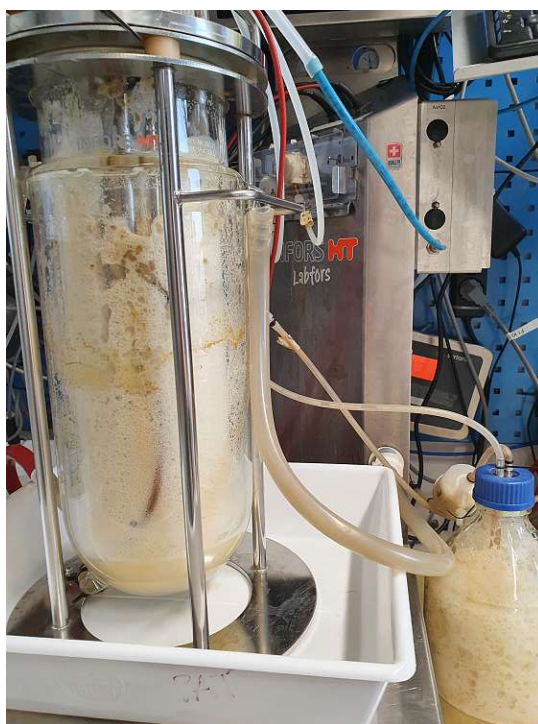
Figure 3.2: End of process through over-foaming of reactor and consequently loss of broth
