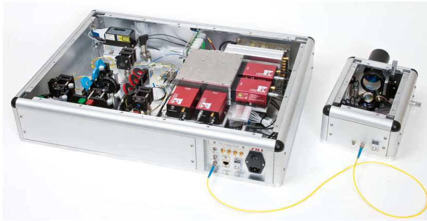
Figure 4.3: AIT-EPR-S405 QKD lab prototype used for research and teaching.
