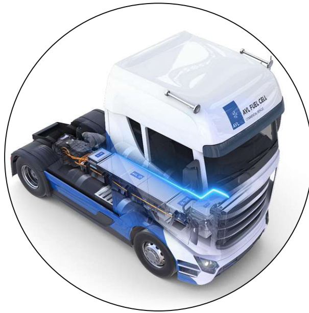
Figure 1.2: Prototype of the 42-ton fuel cell electric truck under development within the Austrian research project FC4HD.
