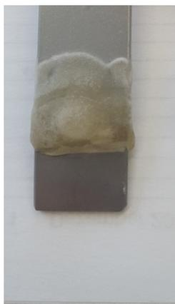
Figure 18: A prepared coupon, which can be used for EIS measurements.
