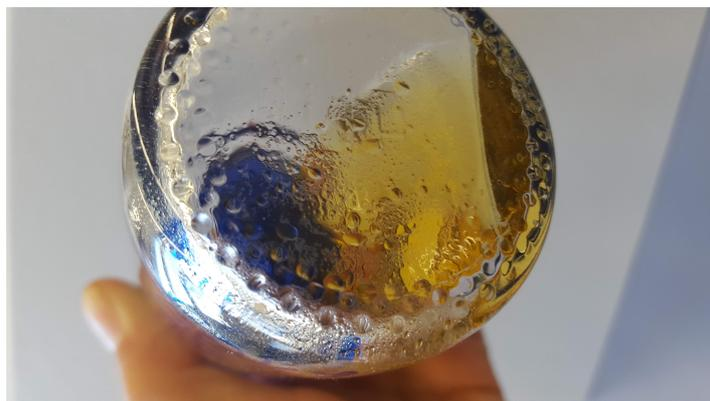
Figure 76: Inhibitor D mixed into methanol.
