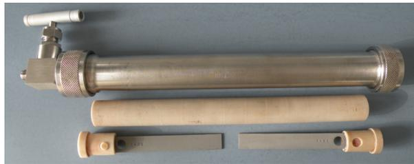
Figure 13: Components of an autoclave and the metal coupons on the sample holder.
