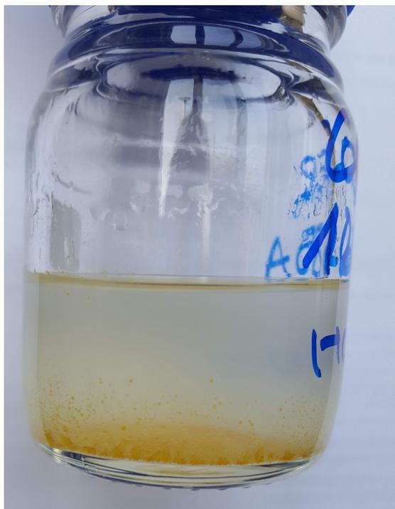
Figure 75: Inhibitor D mixed into hydrochloric acid.
