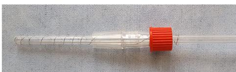
Figure 20: Platinum wire counter electrode for polarization curve measurements.
