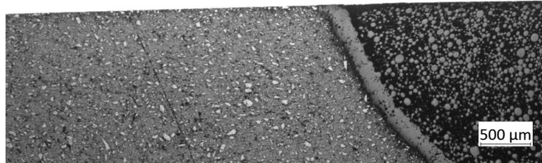
Figure 71: Metal coupon under the microscope after finishing experiments. The coupon is shown as white, lighter grey part is the resin for embedding and the darker grey area is the acrylic resin.
