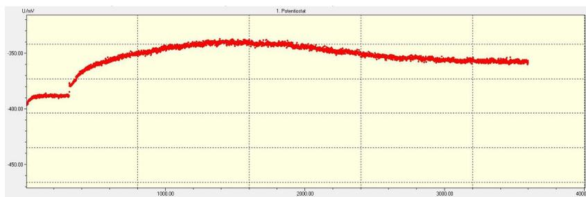
Figure 89: OCP curve in 0.1% Inhibitor I at 50°C.
