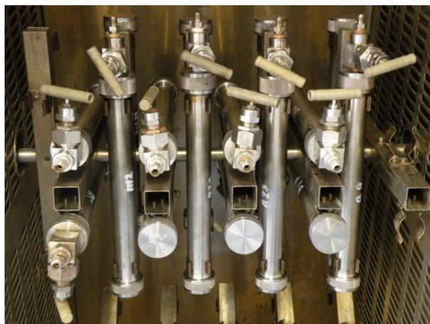
Figure 14: Autoclaves placed on the wheel apparatus.
