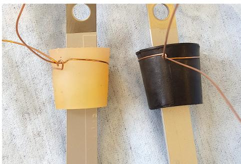
Figure 19: Electrodes mounted in conical frustum shaped rubber.
