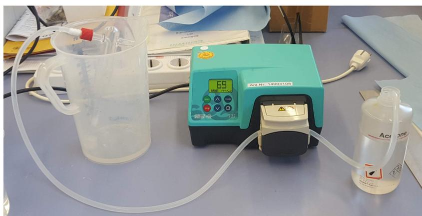
Figure 22: Cleaning gas washing bottle head with acetone using a pump.
