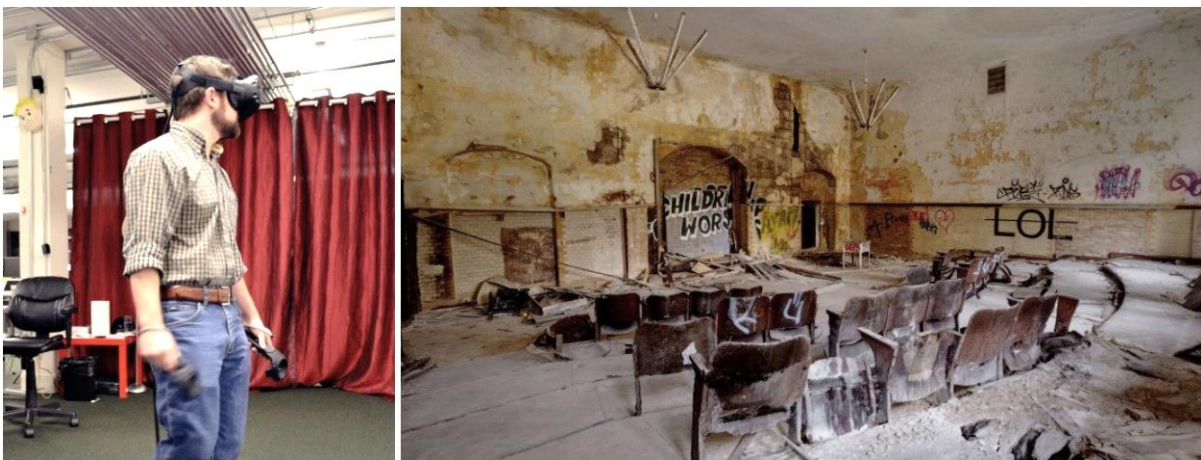
Figure 13. photogrammetry scan in VR, accomplished by company REALITIES: on the left: VR user with HTC Vive. on the right: Photogrammetric scan of existing contexts inside of VR. (@Lang)
