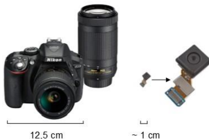
Figure 28. size comparison a DSLR (Nikon D5300) and a smartphone camera module (with 4x zoom in)
