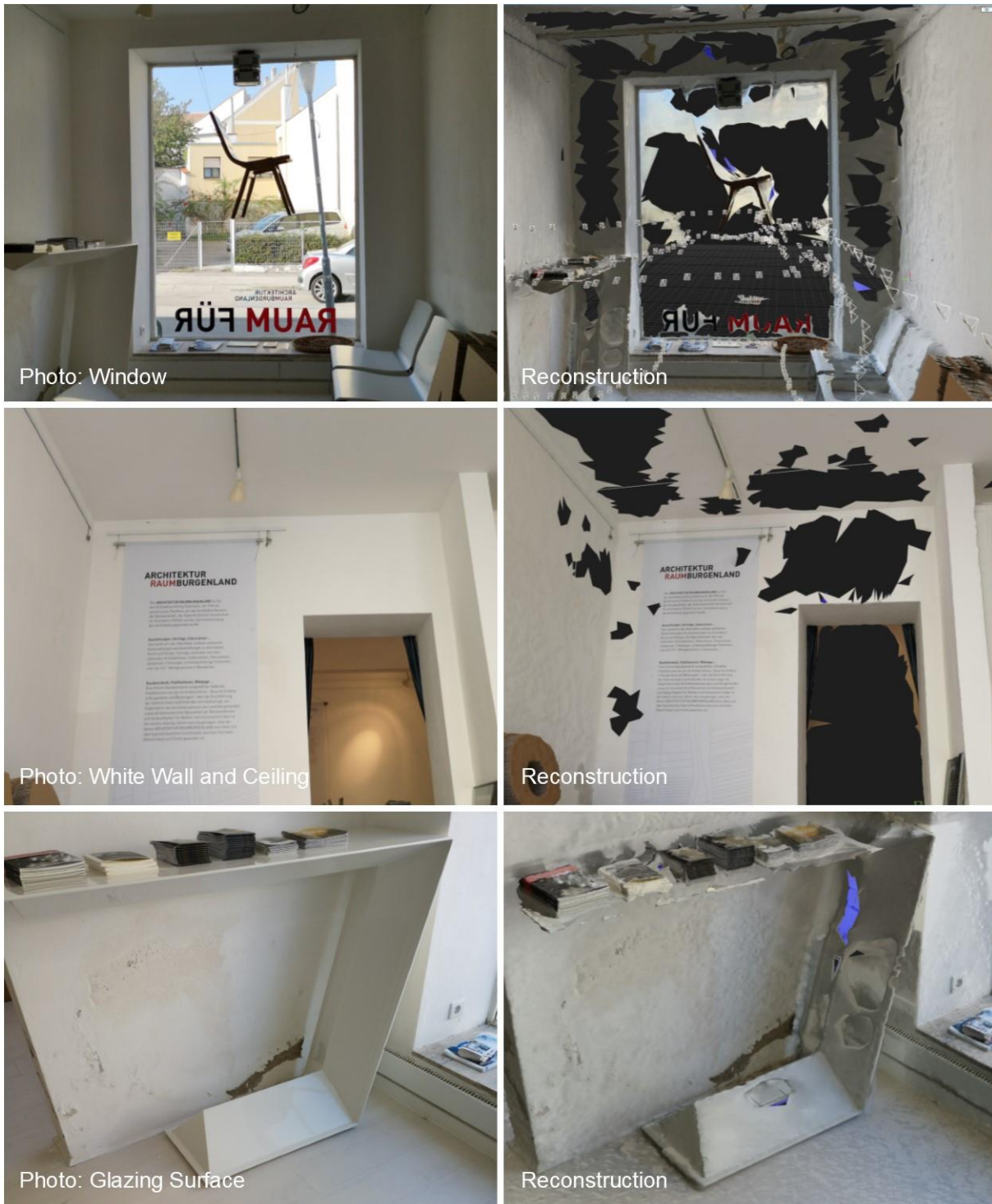
Figure 85. comparison of real on-site photo and photogrammetric reconstruction of the gallery
