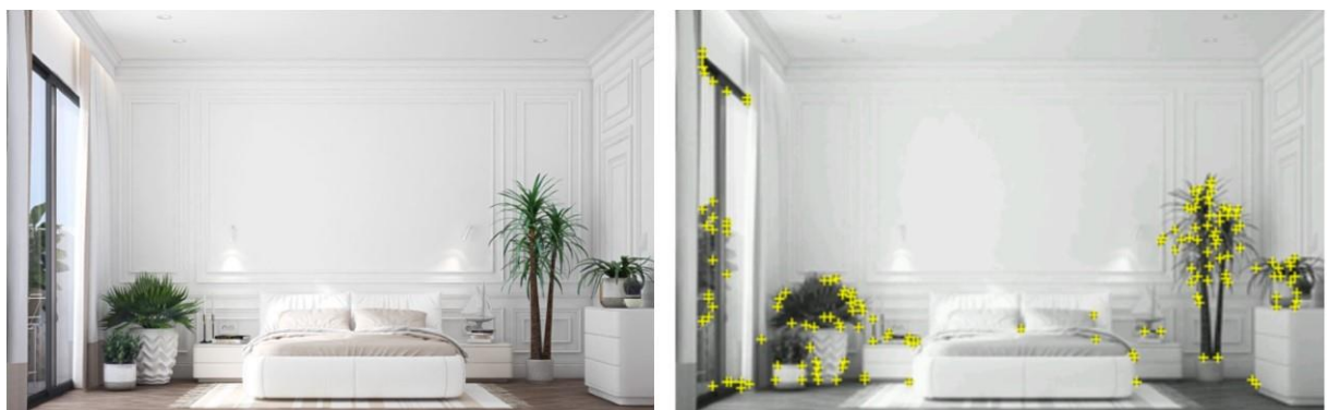
Figure 36. feature detection of monotonous, flat surface: less or none feature could be detected from this type of surface
