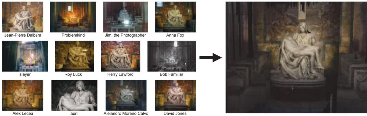
Figure 33. reconstructed 3D model: created from different random internet images
