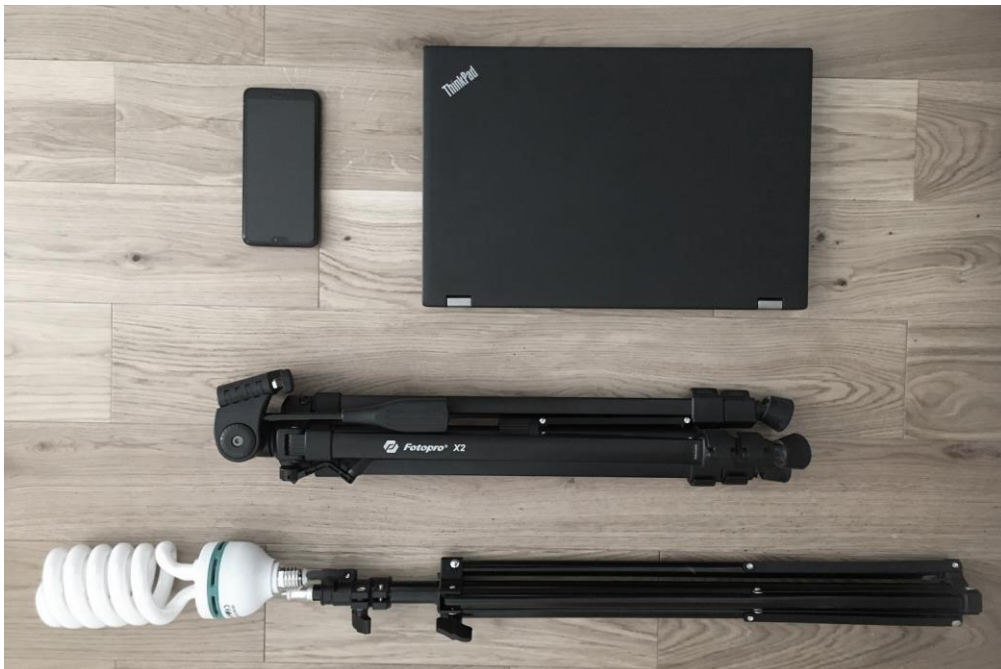
Figure 77. equipment of photogrammetry scan: smartphone Huawei p20 pro, laptop (Lenovo P50), tripod and studio light with stand
