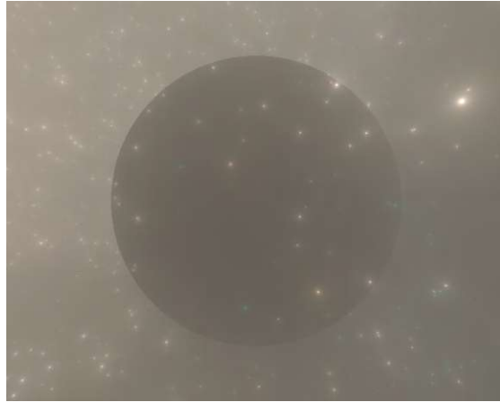
Figure 3.7: A scene rendered with VPL. The singularities in the medium can be seen as there are not enough point lights to illuminate the scene evenly. Source: [NNDJ12b]
