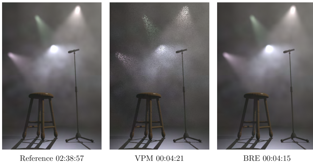
Figure 3.2: A comparison of VPM, the BRE and a reference solution that was rendered with VPM and a small step size. The render time is provided in hh:mm:ss. Source: [JZJ08]
