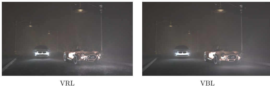
Figure 3.11: A comparison of VRL and VBL. Both of these images were created within the same render time (186 seconds for volume to volume events, 363 seconds for volume to surface events). Source: [NNDJ12a]
