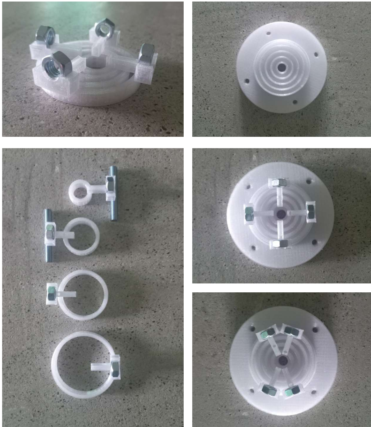
Figure 120: Node connector A. Assembly of a 3d printed, prototype.
