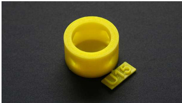
Figure 98: 3d printed node-connector.
