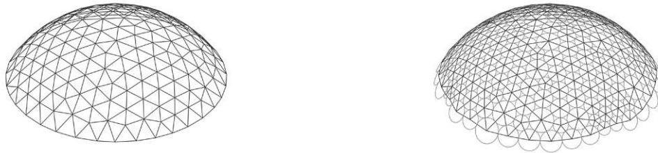
Figure 30: Near equilateral triangular mesh topology optimization to hold a dense circle packing using Kangaroo2.
