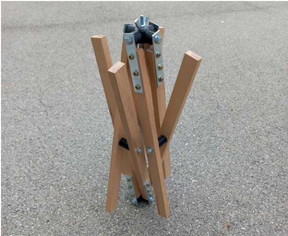
Figure 112: Bracing node prototype. Contracted (left) and deployed (right).
