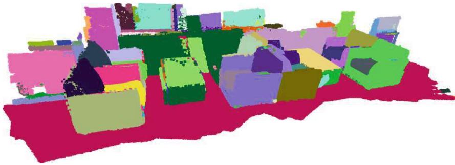
Figure 3.1: Scene 286 from the SceneNN dataset reconstructed as a point cloud using our framework, and visualized with flat rendering in Open3D. Point colors correspond to global segment labels.
