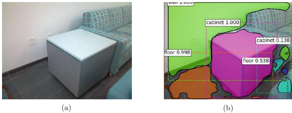
Figure 3.9: Example of instance-aware semantic segmentation on a single video frame, as performed by Mask R-CNN Benchmark. Subplots show RGB input on the left and the segmentation result on the right. Results are visualized with colored segmentation masks, bounding boxes, and class labels.
