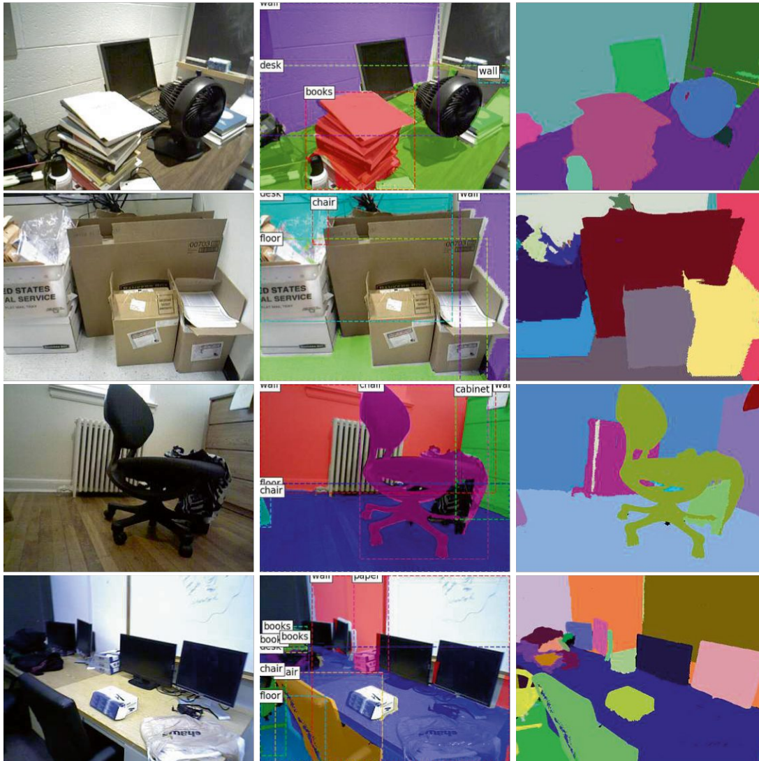
Figure 4.3: Examples of initial training set images with annotations, as shown in the center column. Each annotation consists of a segmentation mask, bounding box, and class label. For visualization purposes, masks and bounding boxes are colored with random colors. The original RGB camera frames (left column) and 2D instance segmentations (right) are provided for reference. Instance segmentations are rendered from ground truth meshes with a unique, random color per instance.
