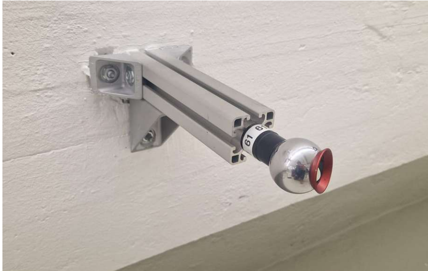
Figure 3.5: RRR in a magnetic console in the measurement laboratory
