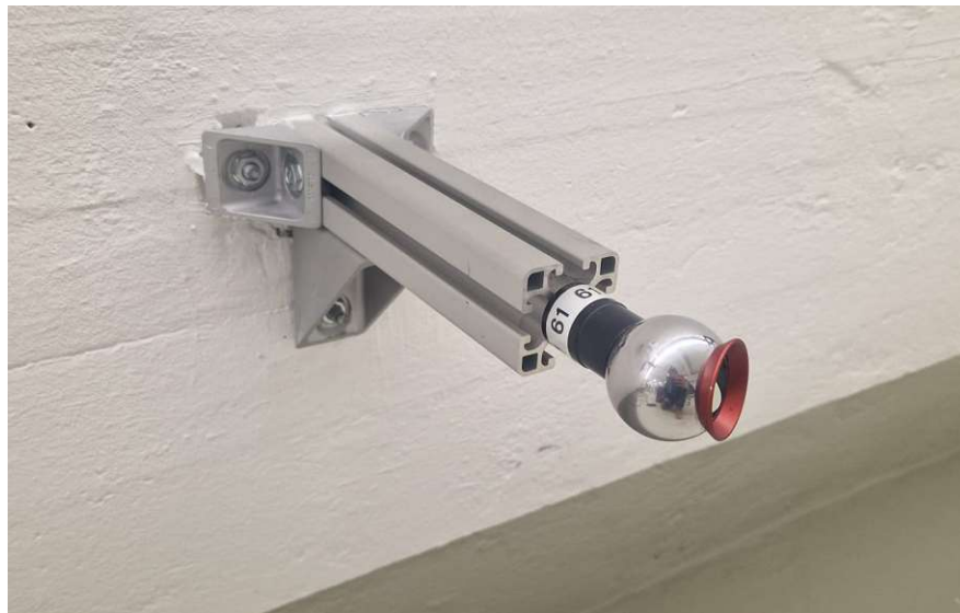
Figure 4.3: RRR in a magnetic console in the measurement laboratory
