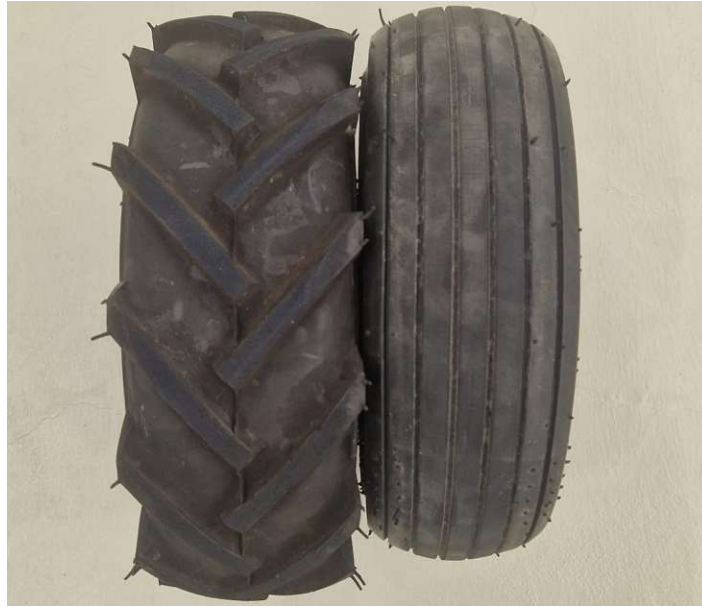
Figure 3.3: Comparison of the original lugged off-road tire (left) and the smooth aftermarket tire which was used for this thesis (right)
