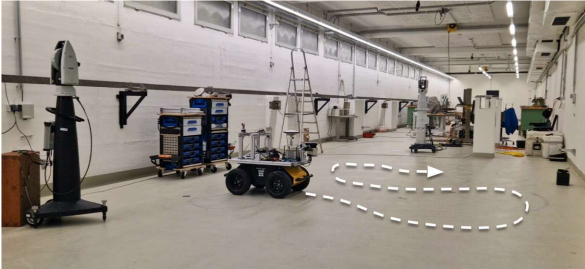
Figure 4.1: Overview of the measurement laboratory with the two laser trackers and the Husky A200 with an illustrated driving path used during the experiments
