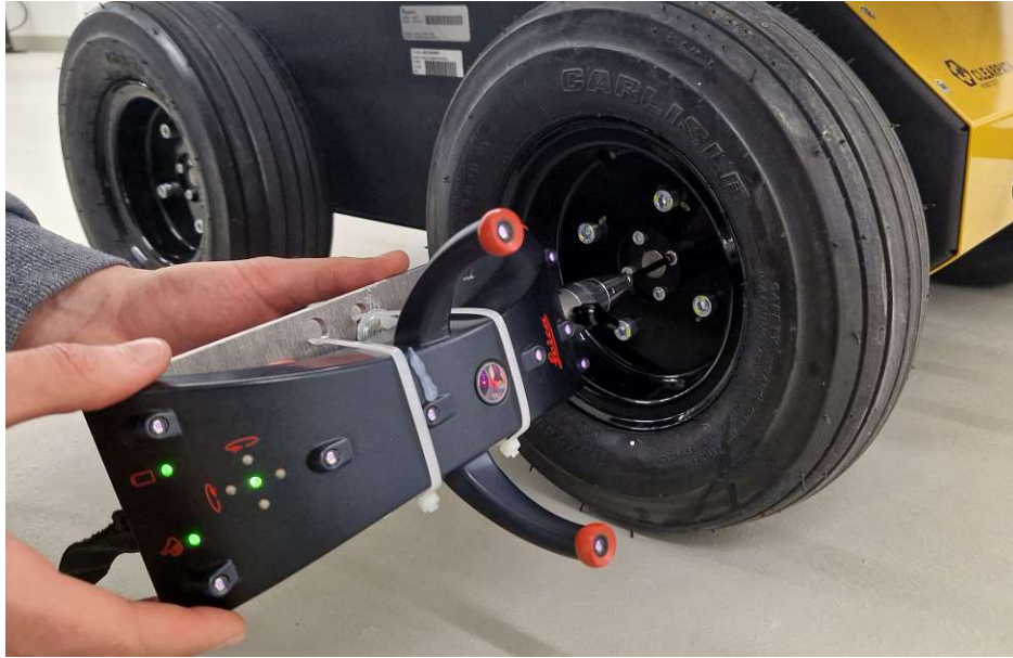
Figure 6.2: Measuring process of the wheel hub screw heads for the body frame realization
