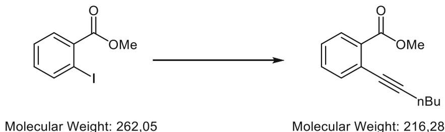
The catalyst Pd(PPh<sub>3</sub>)Cl<sub>2</sub> (130 mg, 0.01 eq) and CuI (80 mg, 0.03 eq) were suspended in 20 mL dry Et<sub>3</sub>N and methyl orthiodobenzoate (5 g, 2.8 mL, 1 eq) was added to the yellow suspension. The color changed to brown and stirring continued for 1 h. The flask was cooled to 0 °C and 1-hexyne (2.35 g, 3.27 mL, 1.5 eq) was added over the course of 10 min.
