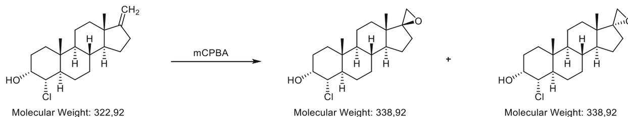
The substrate (350 mg, 0.81 mmol) was dissolved in 7 mL chloroform and 5 mL pH 7 phosphate buffer was added. Under vigorous stirring, mCPBA (250 mg, 70 % in benzoic acid, 1.0 mmol, 1.25 eq) was added. After 90 min, TLC showed complete conversion and the reaction mixture was diluted with DCM and water. The phases were separated and the organic phase was washed with sat. aq. NaHCO<sub>3</sub>, water and brine. After drying over sodium sulfate, the volatiles were evaporated.
