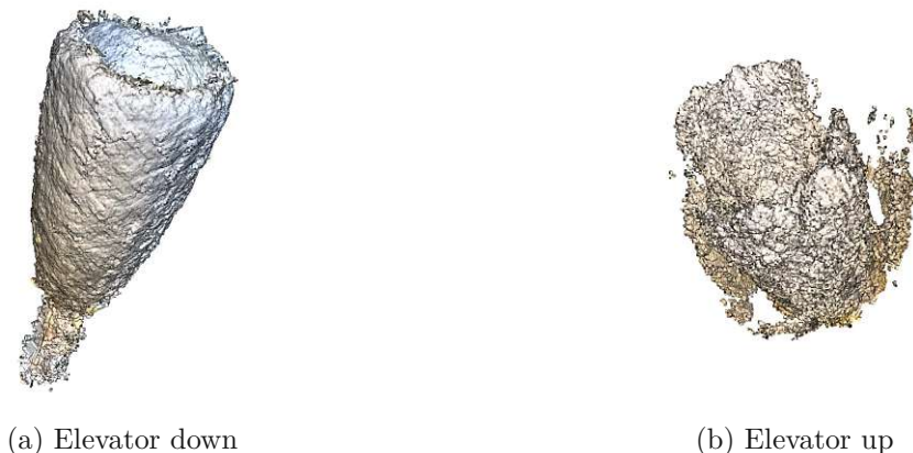
Figure 4.6: Results of 3D object reconstruction on the matte glass with RTAB-Map visual only
