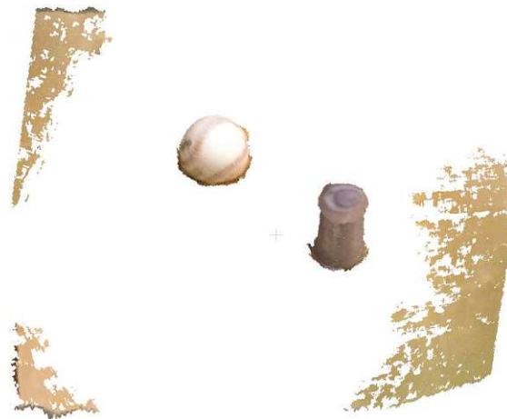
Figure 3.3: Finished reconstruction of the baseball+canister test case with RTAB-Map visual only and camera lift down
