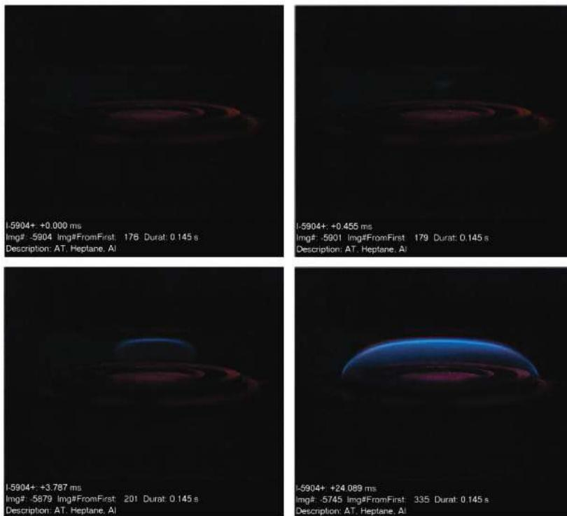
Figure 5.18: Autoignition event recorded with the high-speed camera. The fuel is prevaporized n-heptane at 533 K.
