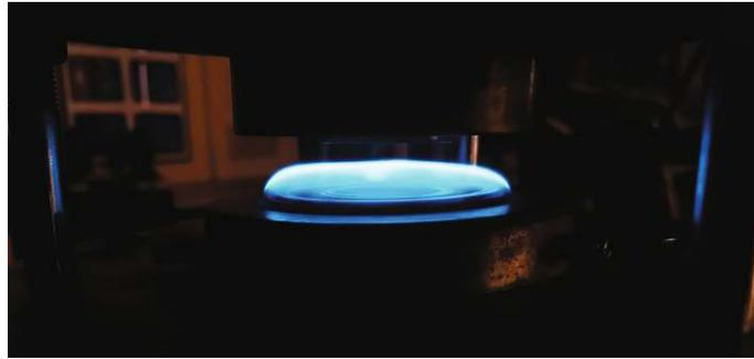
Figure 5.7: Counterflow burner in gaseous configuration (left) and stabilized, non-premixed propane flame (right) during an experiment to determine the extinction strain rate.
