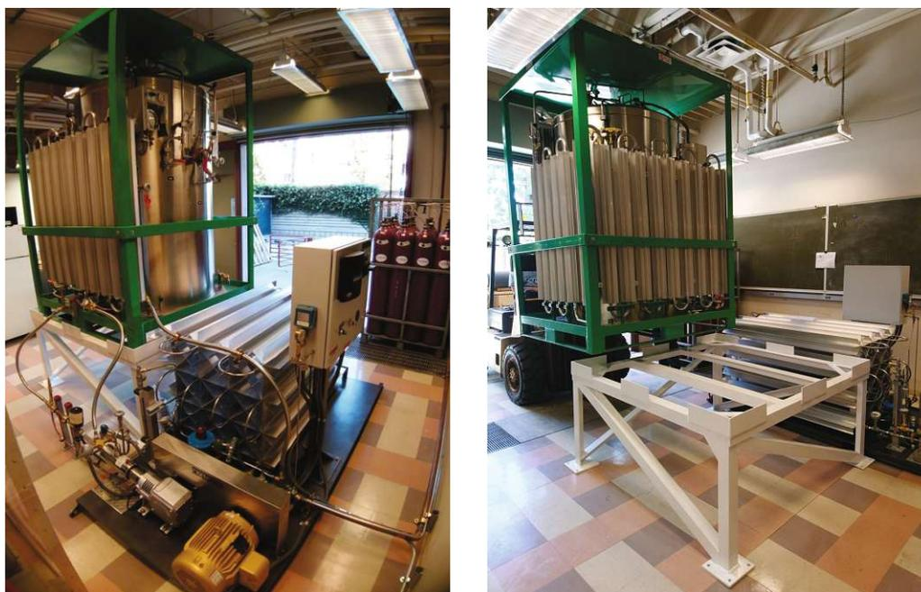
Figure B.12: Nitrogen Supply System - Back view of the system showing the cryogenic pump together with its actuating motor (left) and moving the tank for refilling (right).
