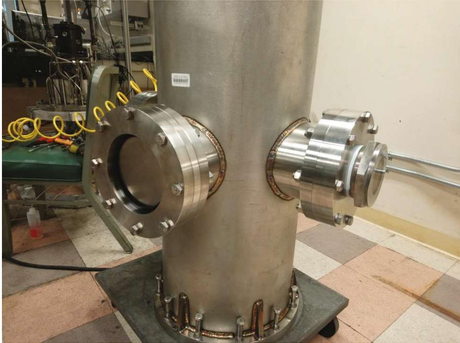
Figure 4.5: Pressure chamber hull showing one viewport covered up with a round stainless steel plate and another one with a sight glass installed.
