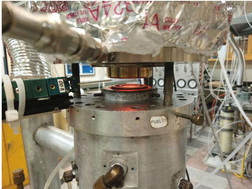
Figure C.1: View of the fuel duct during an ongoing autoignition experiment with inserted thermocouple and the oxidizer stream at around 1100 K.
