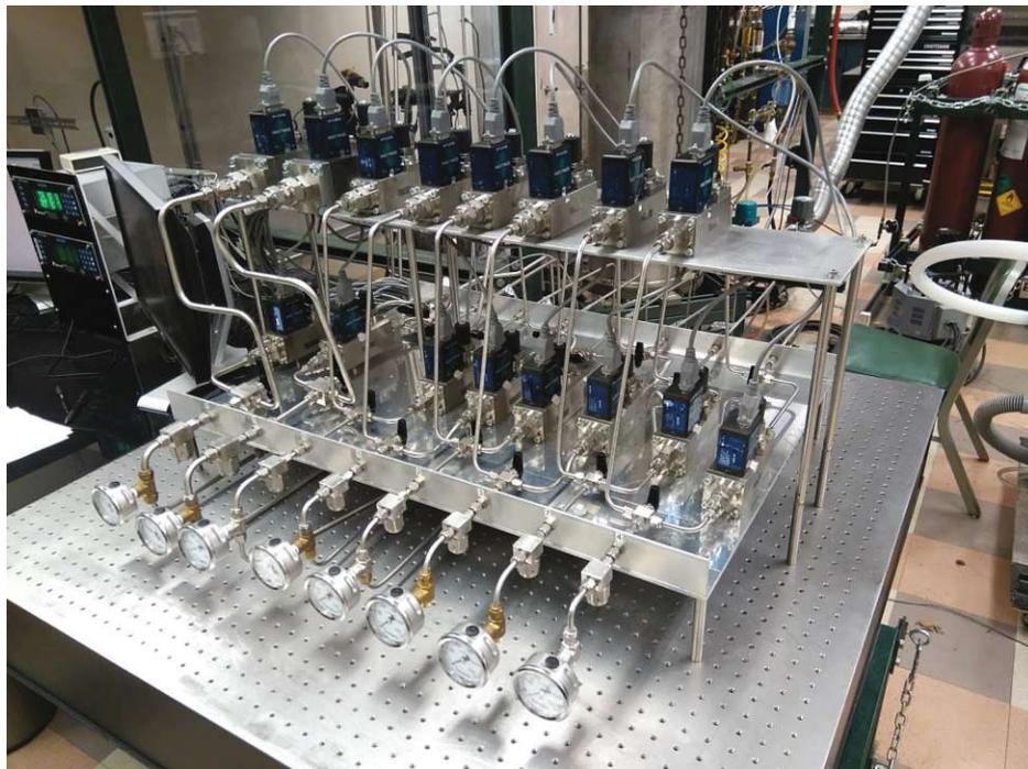
Figure 4.4: Flow control stand with the high pressure set of mass flow controllers in parallel on top of the low pressure set in its idle state.
