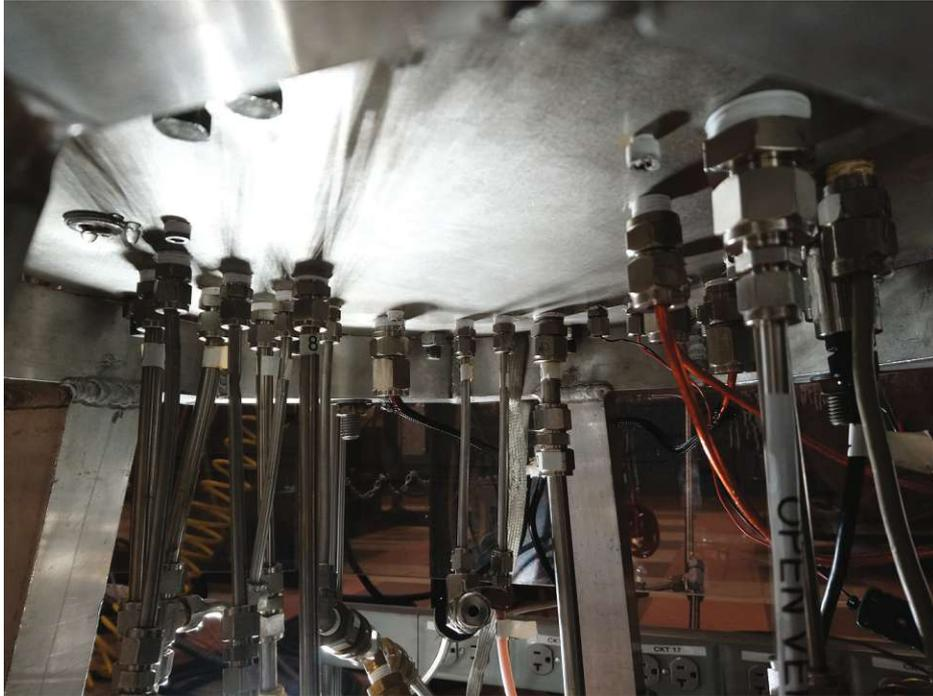
Figure B.5: High Pressure Combustion Experimental Facility - View of the bottom plate during pressure testing, with droplets of water forming on fittings showing leakage.
