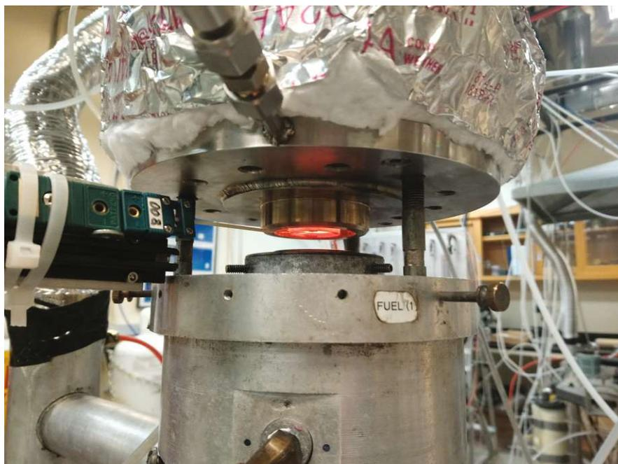
Figure C.2: View of the oxidizer duct during an ongoing autoignition experiment with inserted thermocouple and the oxidizer stream at around 1100 K.
