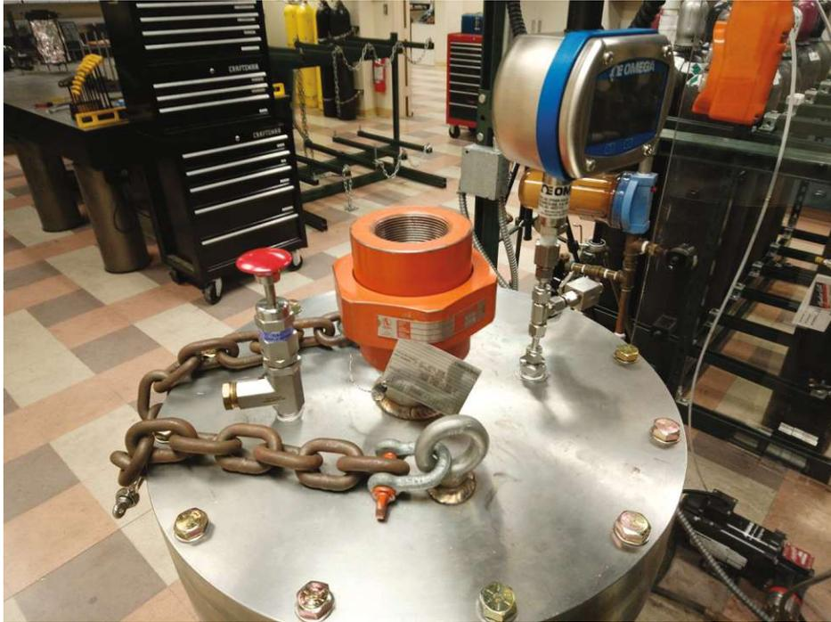
Figure 4.7: Pressure chamber's top plate bearing a pressure relief valve, burst disc assembly, ball valve for venting, pressure gauge and eyes for connecting to the electric hoist.
