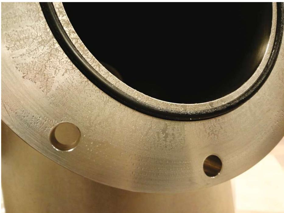
Figure B.6: High Pressure Combustion Experimental Facility - Residual water on o-ring sealed surface after pressure testing with water.
