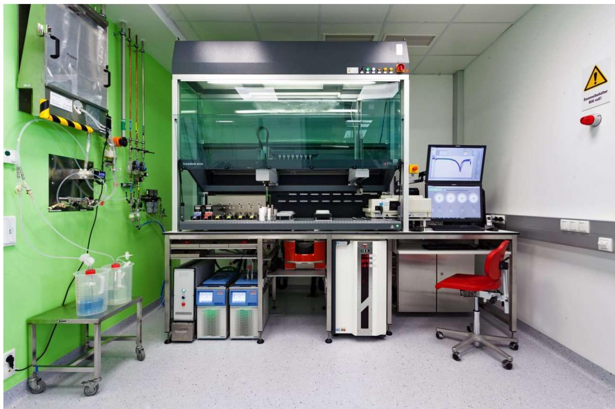
**Figure 2.** The used mini-bioreactor system (bioREACTOR8; 2mag AG), and the experimental setup (Boehringer Ingelheim RCV GmbH & Co KG).
