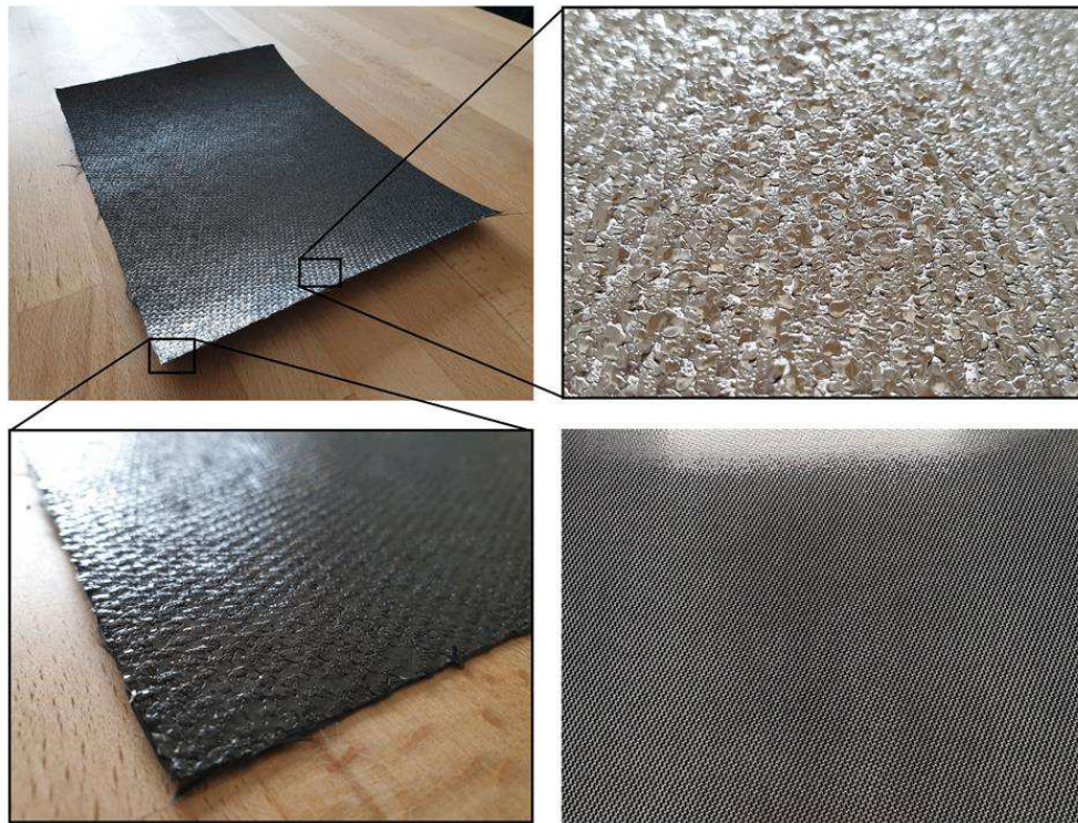
Fig. 29 CF-polymer powder-semipreg (top left, top right and bottom left), and compression moulded laminate therefrom (bottom right).
