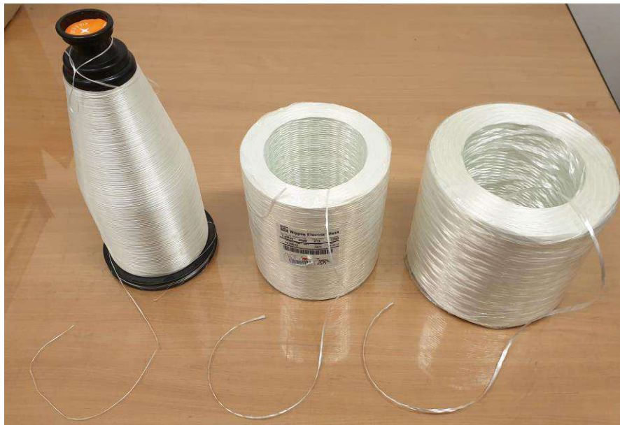
Fig. 2 Left to right: E-glass fibre yarn 300 Tex, E-glass fibre roving 1200 Tex, E-glass fibre roving 2400 Tex. Yarn bobbin is unwound by external pull, roving bobbins by internal pull.
