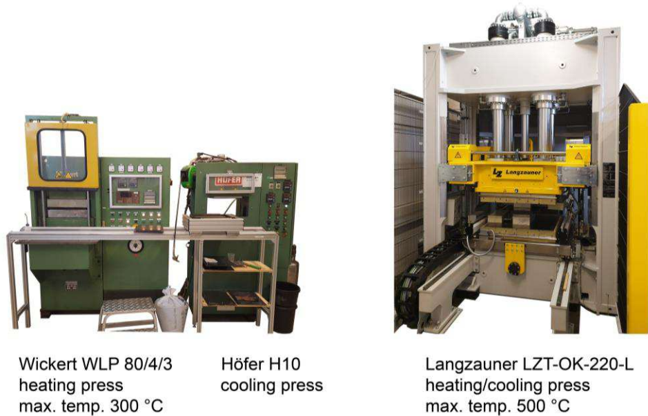
Fig. 33 Static heating and cooling presses utilised in the experiments.
