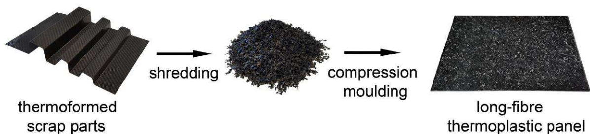
Fig. 31 Recycling route for TPCL via shredding and compression moulding
