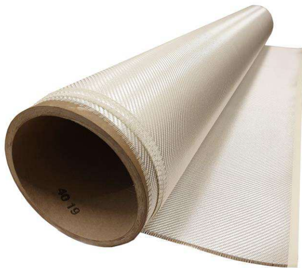
Fig. 5 Glass yarn fabric 50'' (Gividi Fabrics VR48 2/2 twill) based on 68 x 3 Tex yarns with an areal weight of 290 \text{ g/m}^2 and thread count of 7/cm.
