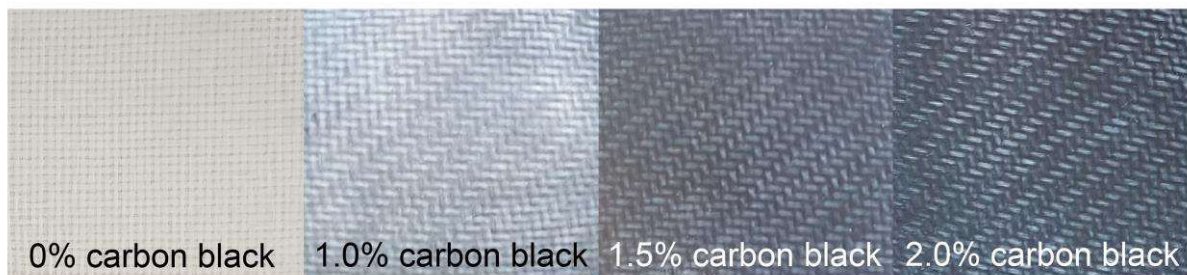
Fig. 40 Required amount of carbon black masterbatch to make GF-PP TPCL visually more appealing.
