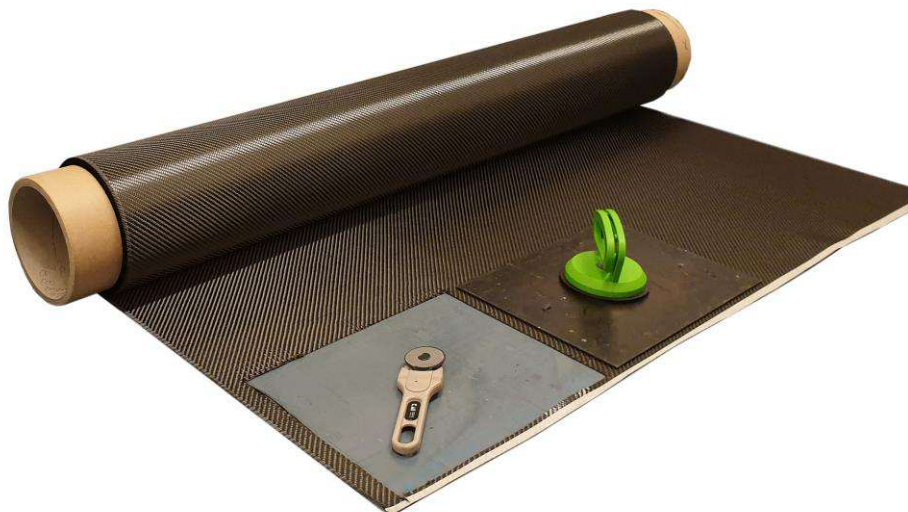
Fig. 7 Carbon fibre fabric 50'' (ECC - Engineered Cramer Composites Style 452 2/2 twill) based on 3K - 200 Tex tows with an areal weight of 200 \text{ g/m}^2 and thread count of 5/cm.
