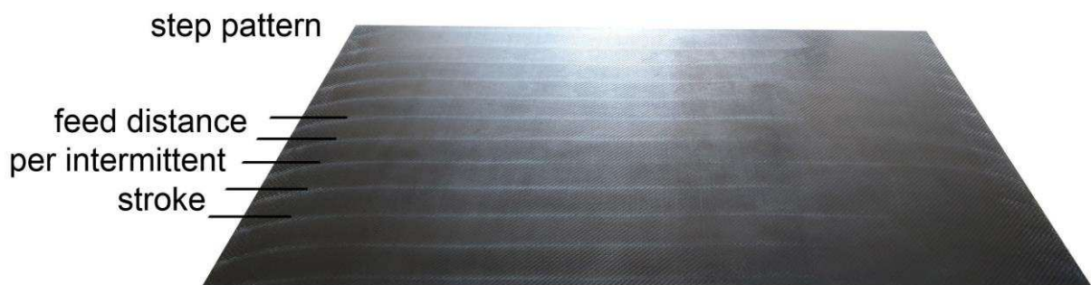
Fig. 28 Step pattern arising from semi-continuous pressing of a 50” wide Tepex ® 202 CF-PA6 TPCL produced by Bond Laminates GmbH.
