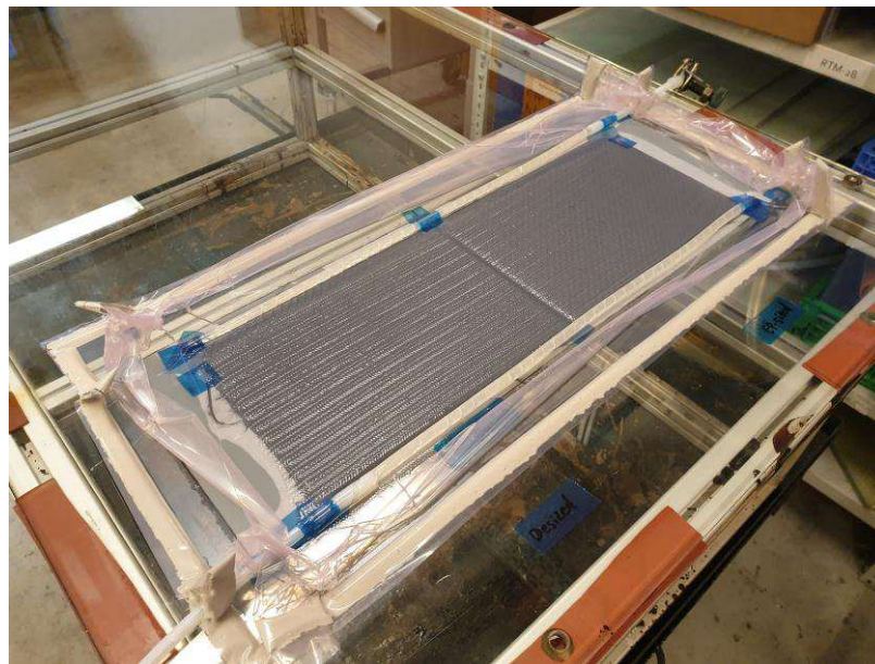
Fig. 34 Vacuum assisted infusion of carbon fibre fabrics with epoxy resin. Resin inlet (left), resin outlet to vacuum pump (right) and infusion lines. Dry CF stack is covered by a peel ply, flow media and the vacuum bagging film (secured by sealant tape).
