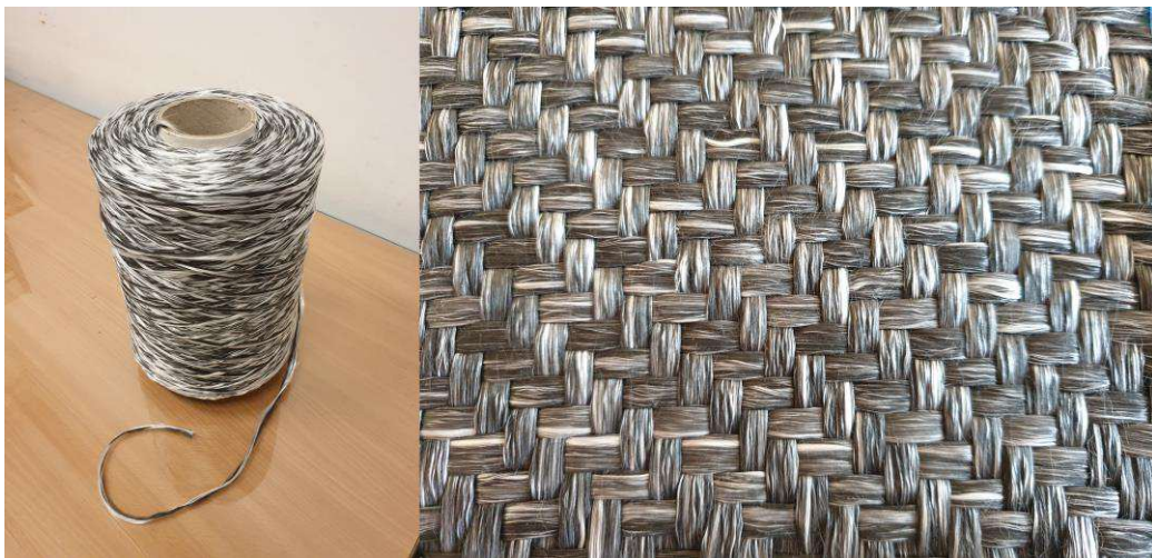
Fig. 30 Commingled GF-PP roving (left) and commingled GF-PP roving fabric (right).
