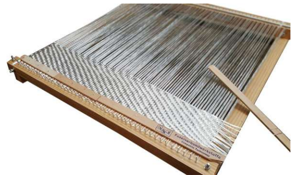
Fig. 1. Loom constructed for manual weaving of PP-compatible rovings.
