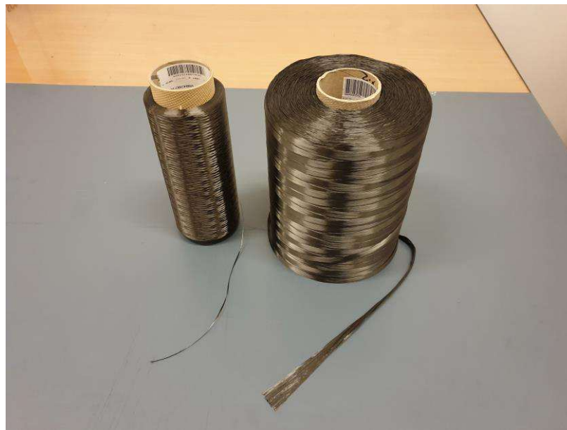
Fig. 3 3K high tenacity (HT) carbon fibre tow (left) and 50K HT carbon fibre tow (right). Both bobbins are unwound by external pull.
