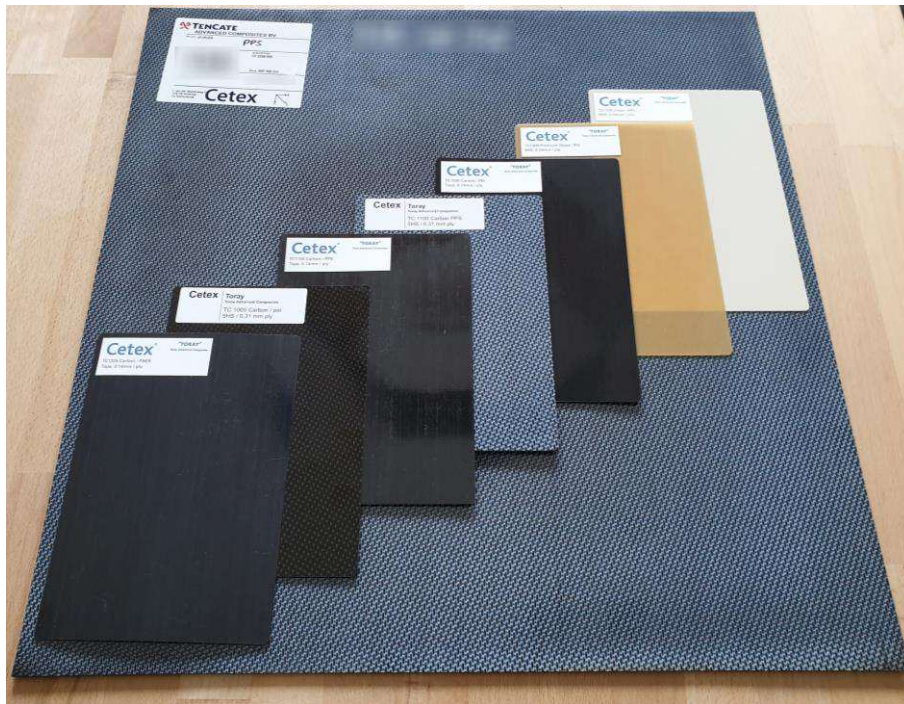
Fig. 27 Cetex ® TPCL consolidated on static presses. CF-PPS fabric TC1100 (large panel background 500 · 500 mm 2 ); TPCL from bottom left to top right: CF-LMPAEK UD, CF-PEI fabric, CF-PPS UD, CF-PPS fabric, CF-PEI UD, GF-PEI fabric, GF-PPS fabric. Samples kindly provided by Toray Advanced Composites.
