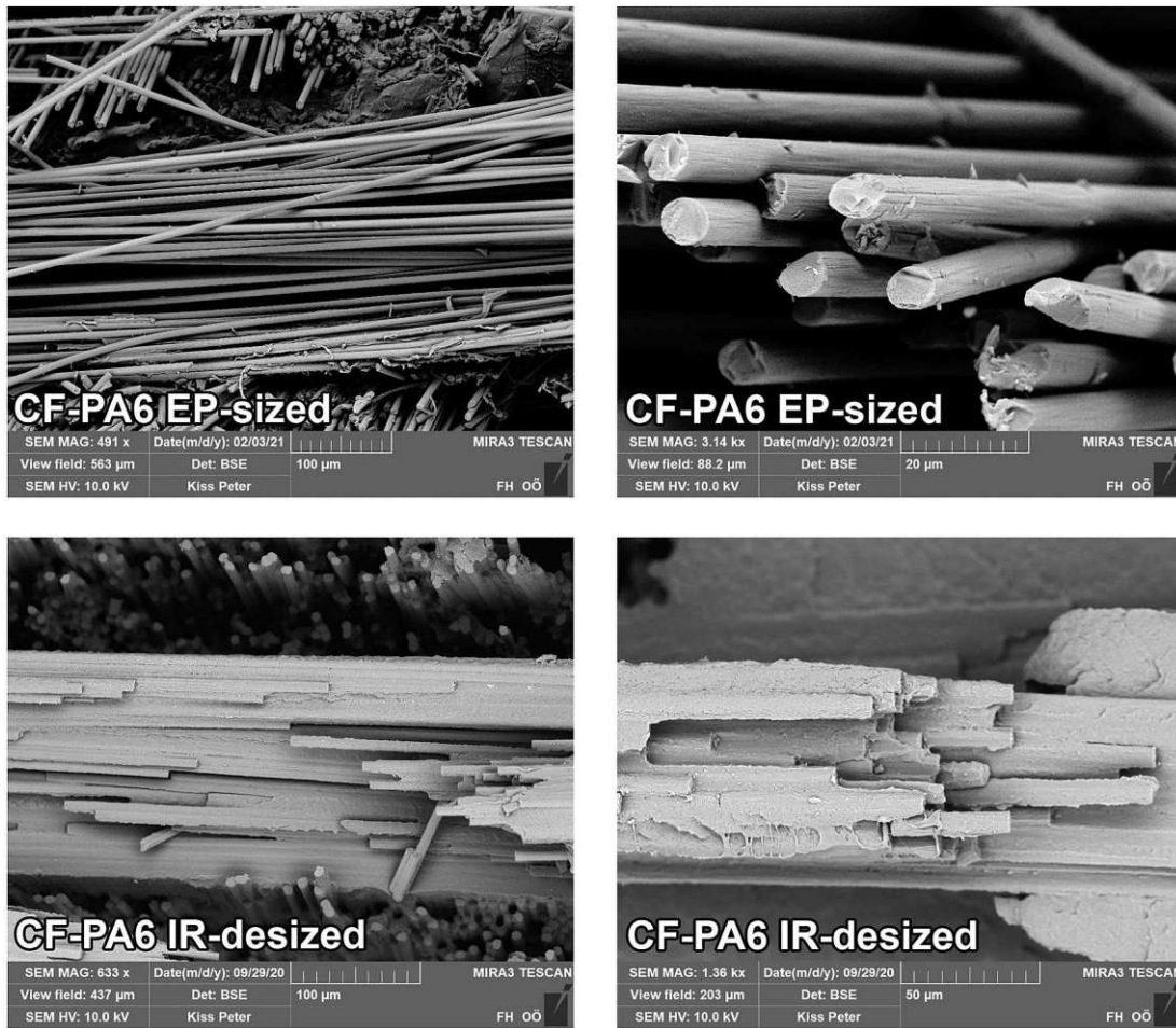
Fig. 8. SEM micrographs of EP-sized CF-PA6 laminate (top) and IR-desized CF-PA6 laminate (bottom). The EP-sizing inhibited wet-out of the fibre bundles resulting in a flexural modulus of 8 GPa and flexural strength of 82 MPa of the laminate. Note, both laminates were moulded with the same parameters.
