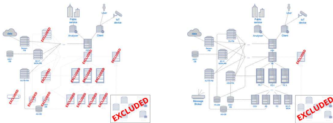
(a) The big picture of the "conventional" system. It excludes all blockchain components, the policy administrator, the policy engines and all validation components.
