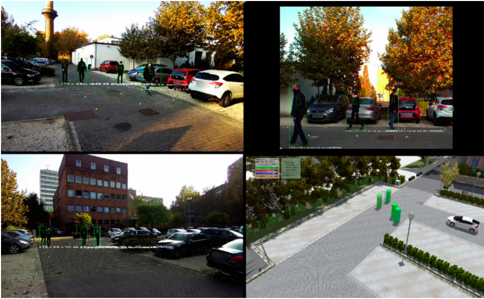
Figure 24. Objects sensed by different sensors of the infrastructure (left) and the vehicle (top-right), respectively, and visualisation of the real-time digital twin (bottom-right) [145].
