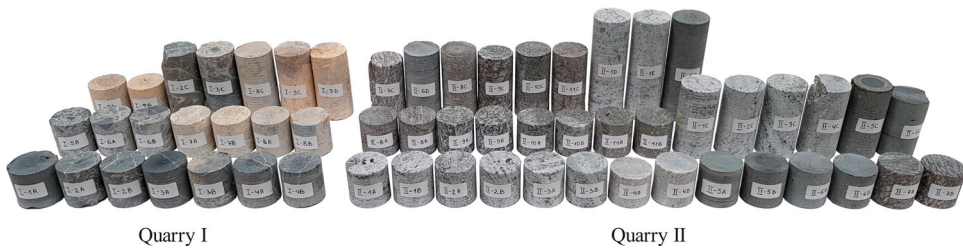
Figure 1. Overview of the produced cylindrical specimens using rock material from two quarries.
