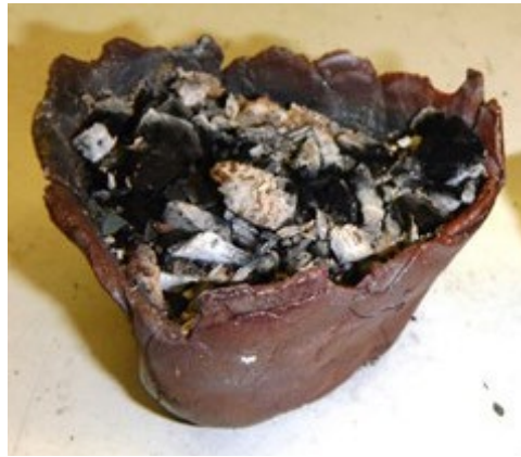
Fig. 2 Self-made clay crucibles after an experiment.
